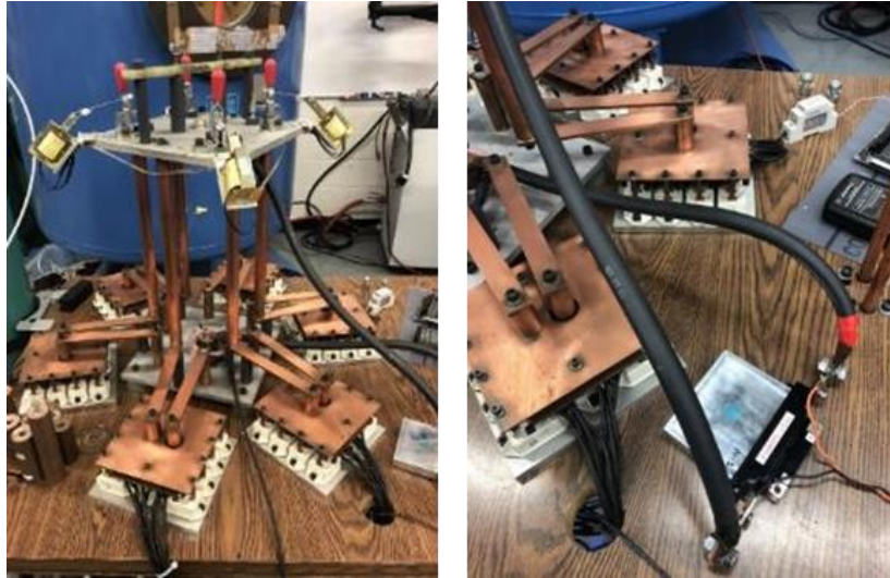
Figure 16. The single pulsed discharge experimental testbed (left) and a Toshiba cell (right) firmly connected using 3/0 copper welding cable and additional bus work attached to the cell.
