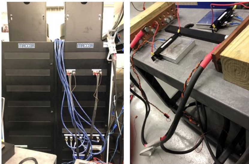
Figure 14. A Maccor cycler used for cell characterization (left) and two Toshiba cells placed on an open-air cart for characterization (left).
