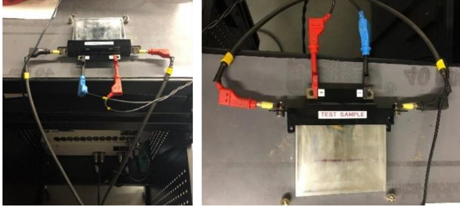
Figure 15. Photographs of the Toshiba cells set up for initial characterization from the PGSTAT302N.
