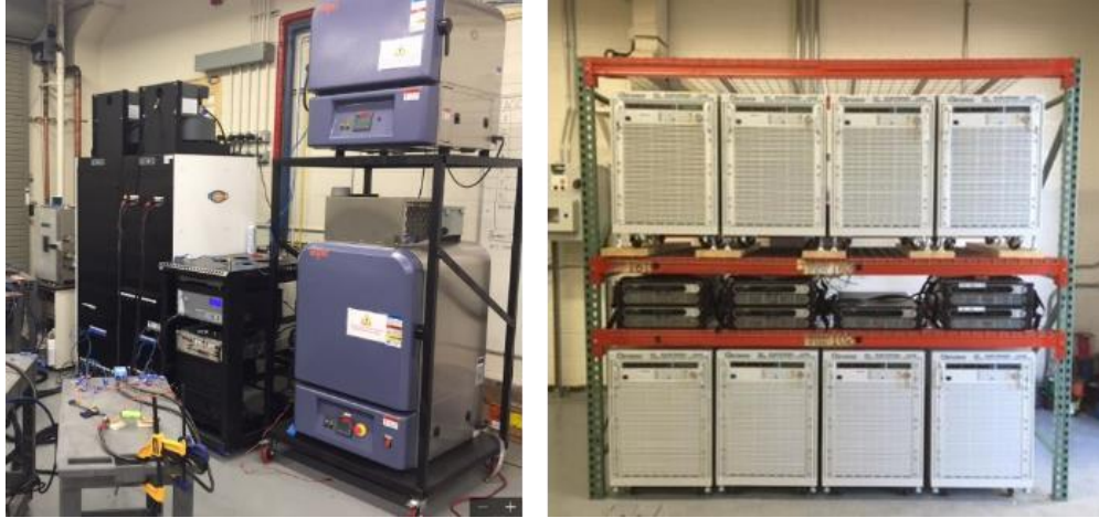
Figure 18. Photograph of the Espec programmable temperature chambers (left) and the power supplies and loads (right).
