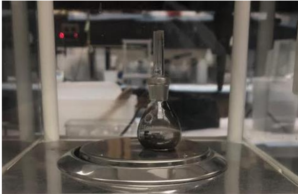
Figure 13: Pycnometer filled with de-aired deionized water and granular samples. Used during liquid pycnometry to determine apparent bulk density for granular samples.
