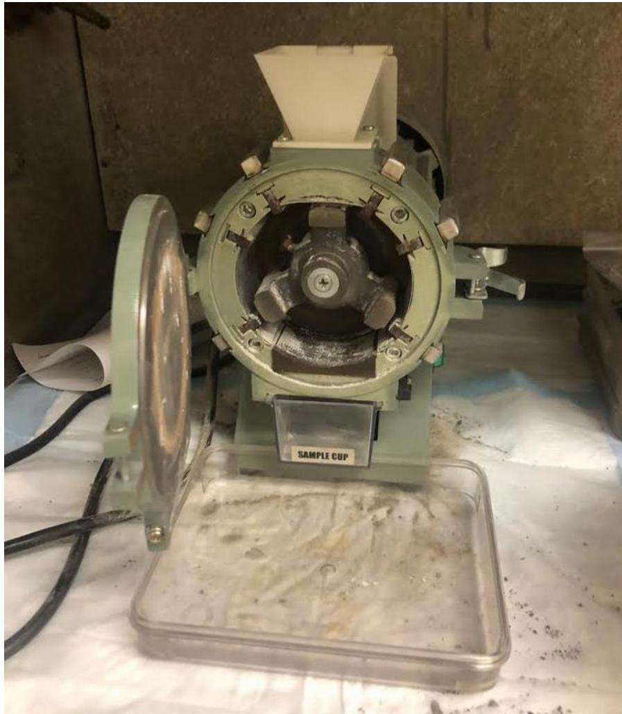
Figure 5: FT-120 grinder used to crush sample pieces into granular sediment
