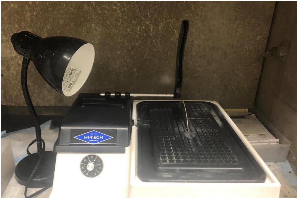
Figure 4: Hi-Tech diamond saw used to cut cores and plugs into cubes and thin slabs
