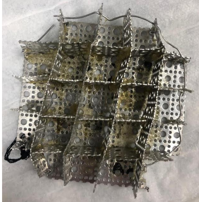
Figure 10: Aluminum rack used during vacuum saturation to keep samples organized
