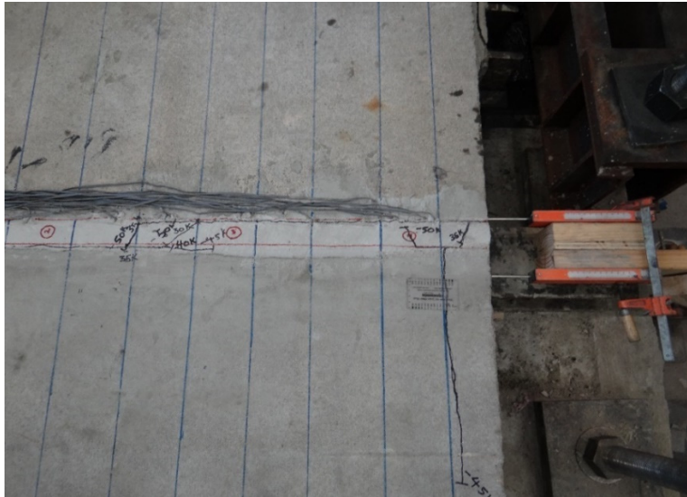
Figure 4-34 Developing some diagonal cracks -50K.
