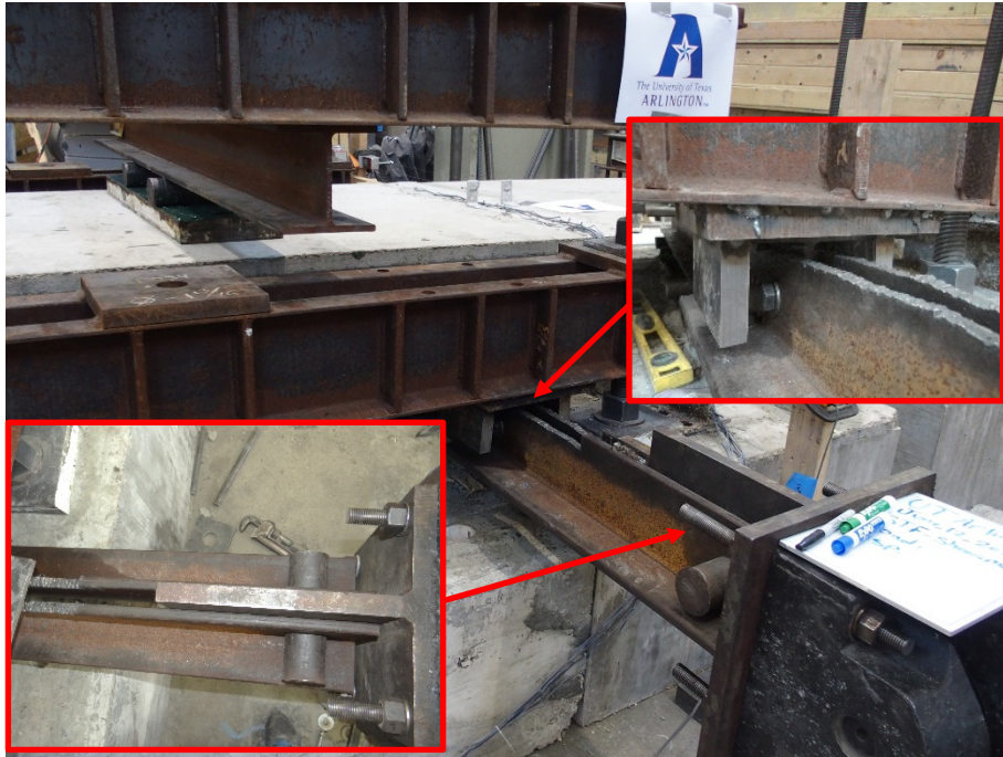
Figure 3-46 Details of connecting the actuator to the specimen.
