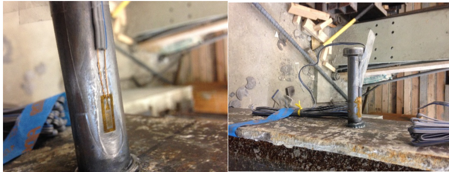
Figure 3-33 Strain gauges installing process on the shear stud
