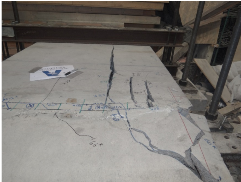
Figure 4-14 Sideview of developing and propagating of cracks at 66 Kips.
