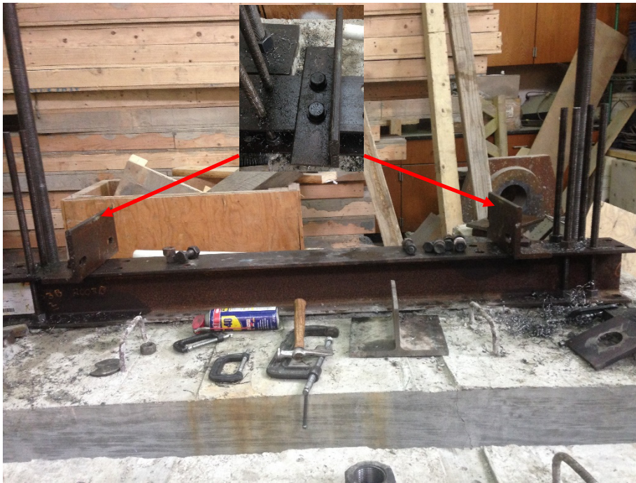
Figure 3-30 Supports at one end of the concrete hollow core planks (Fixed side).
