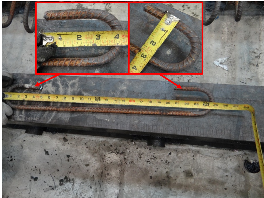
Figure 3-58 Hooked longitudinal rebar and its dimensions.
