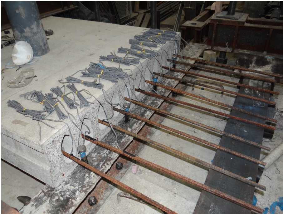
Figure 3-55 Picture of strain gauges locations on the longitudinal rebars and shear studs.
