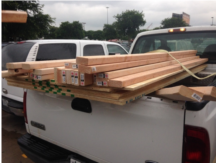
Figure 3-6 Picking up the timber of X-section 4”X2” and plywood of 5/8” thickness.
