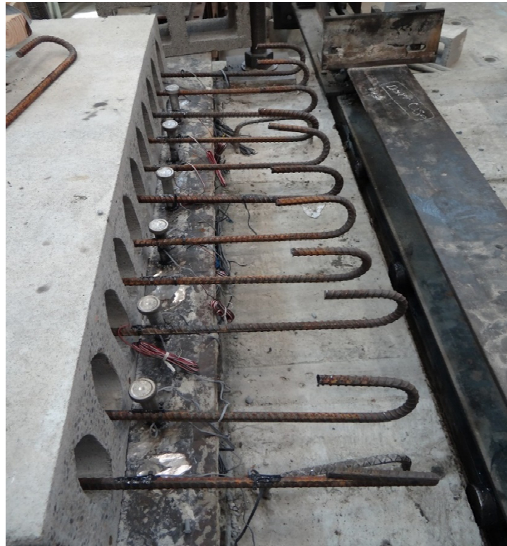
Figure 3-60 Picture of strain gauges on the longitudinal rebars and shear studs.
