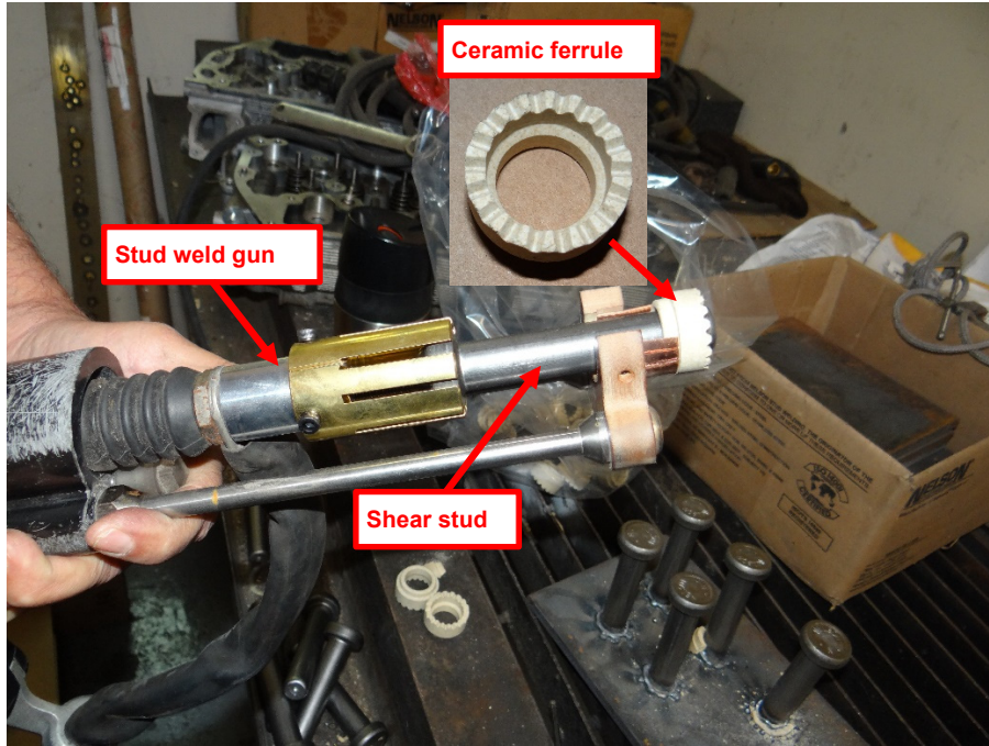
Figure 3-24 Welding equipment; Stud gun; ceramic ferrule.
