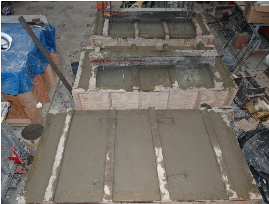
Figure 3-19 The specimens after finishing the casting.
