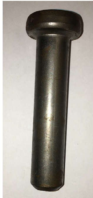
Figure 3-22 Shear stud dimensions in inch; picture of the shear stud
