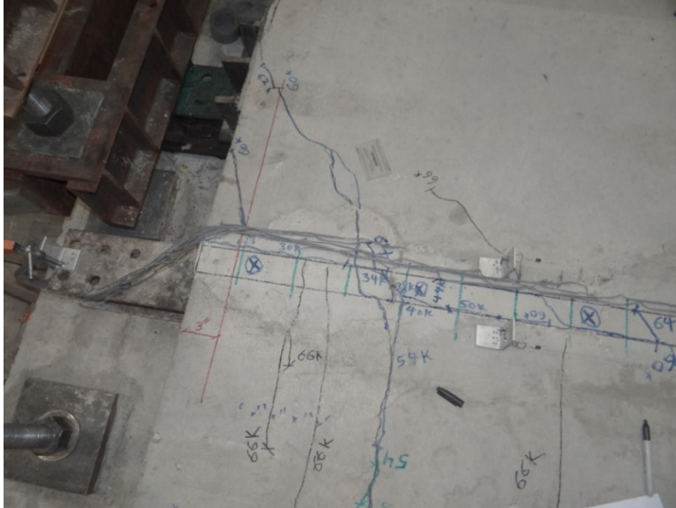
Figure 4- 12 The diagonal crack at 64 Kips.
