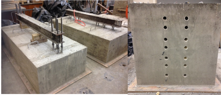
Figure 3-20 The specimens after remodeling the formworks.
