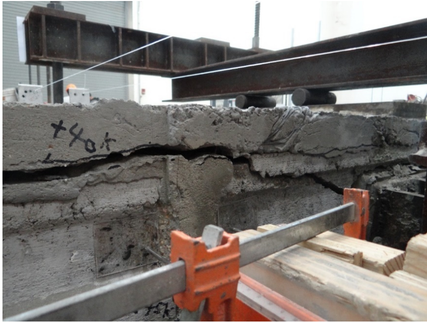
Figure 4-113 Separation between the topping and the planks at (-55 Kips).
