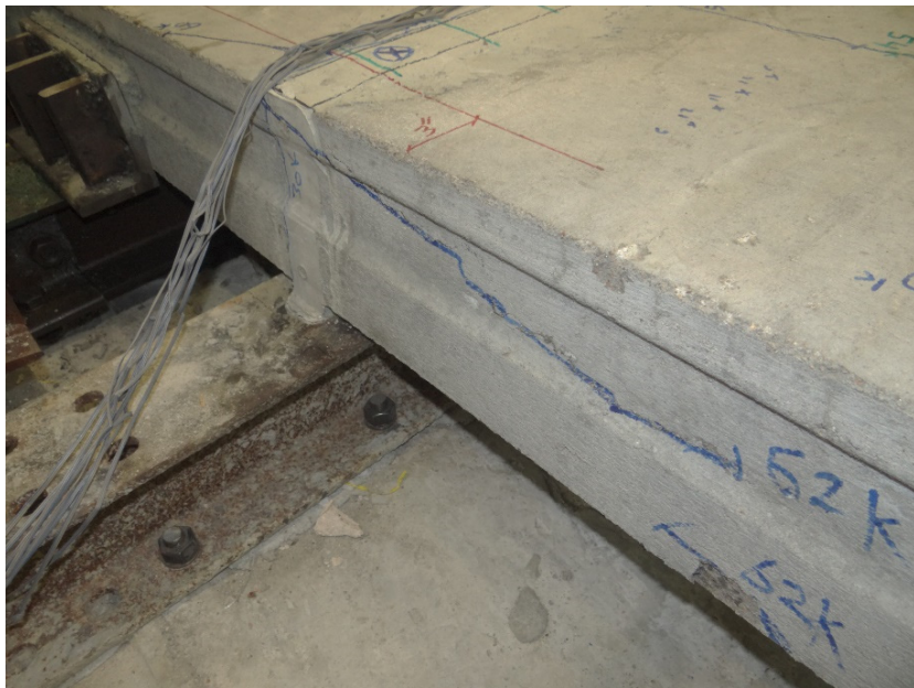
Figure 4-11 Sideview of cracks propagation at 62 Kips.
