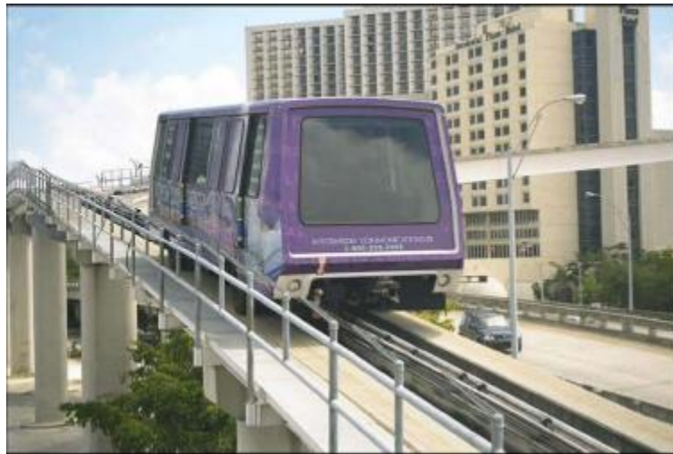
Figure 2. 4 An Automated Guideway Transit (AGT) as downtown people mover in Miami (Source: KFH Group, 2013)
