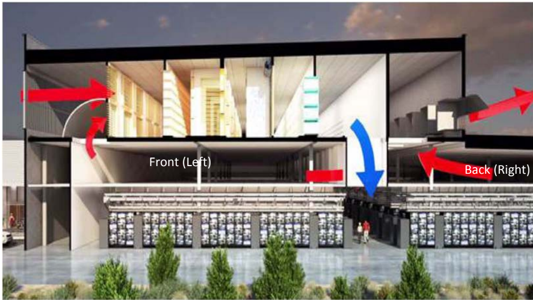
Figure 7-1 Open compute data center airflow path [36]
