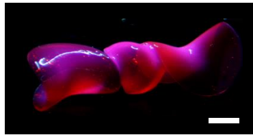
Figure 2-18 Stingray-inspired 3D structure without linkers. The stingray-inspired 3D structure was constructed with the same modules for the body and the pectoral fins used in the structure in Figure 2-15m but without linkers. Although they maintain the designed shape ( K < 0 ), the pectoral fin structures are randomly oriented with respect to the body without linkers. Scale bar, 2 mm.
