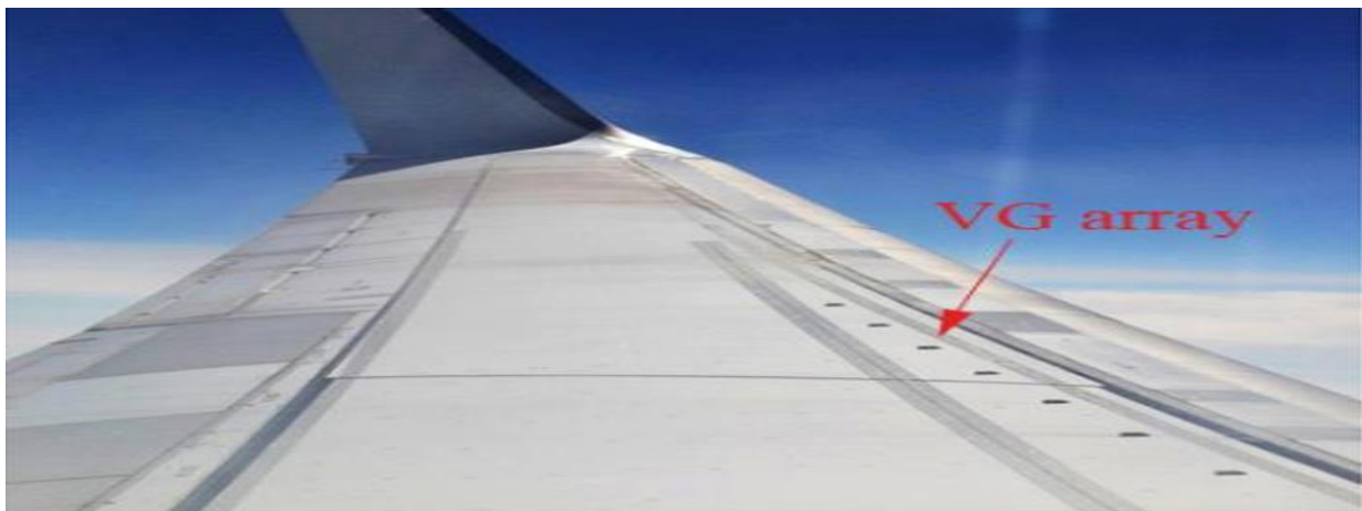
Figure 2. 14 An array of vortex generators on the aircraft wing for shock buffeting control (picture taken on B737-800, operated by Transavia airlines, flying from Barcelona to Amsterdam)
