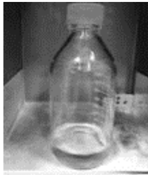
Figure 9: Aging PCB sample immersed in Mineral oil inside a furnace.
