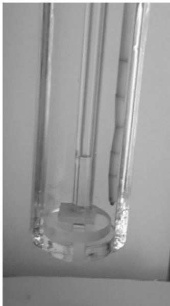
Figure 25: Sample on TMA stage before CTE measurement.
