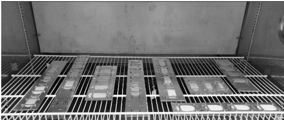
Figure 27: Chamber used for thermal cycling test (top). Samples inside the environmental chamber (bottom).
