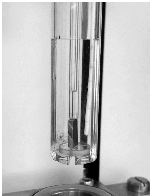
Figure 11: Megtron6 PCB sample mounted on the TMA for testing.
