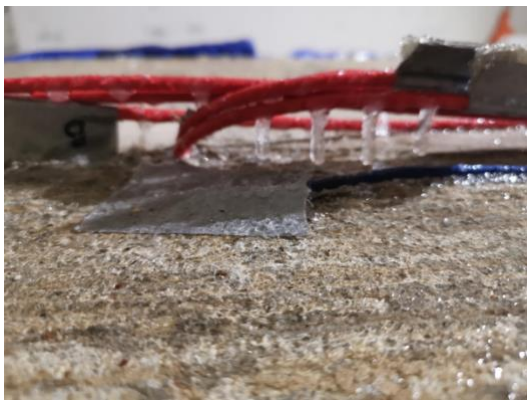
Figure 49. Final slab condition with the formation of glaze after case 1.1 testing
