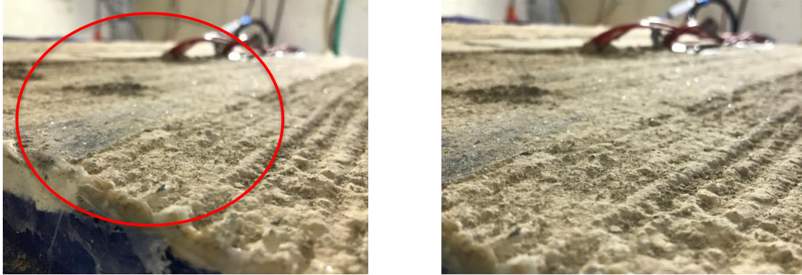
Figure 59. Fine layer of frost on the slab surface
