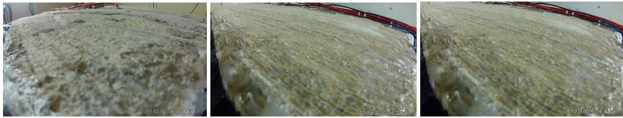
Figure 53. (a): Slab surface under dry conditions (b): Slab surface 20 minutes into misting (c): Slab surface 15 minutes after misting
