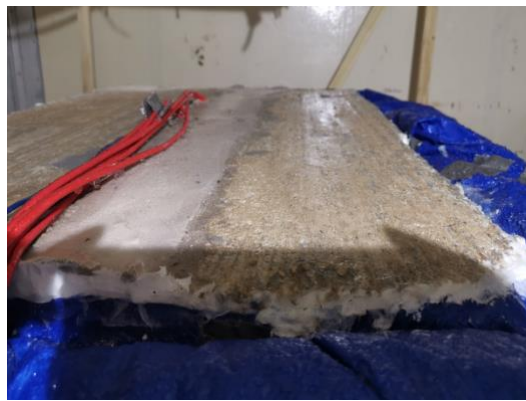
Figure 49. Final slab condition with the formation of glaze after case 1.1 testing
