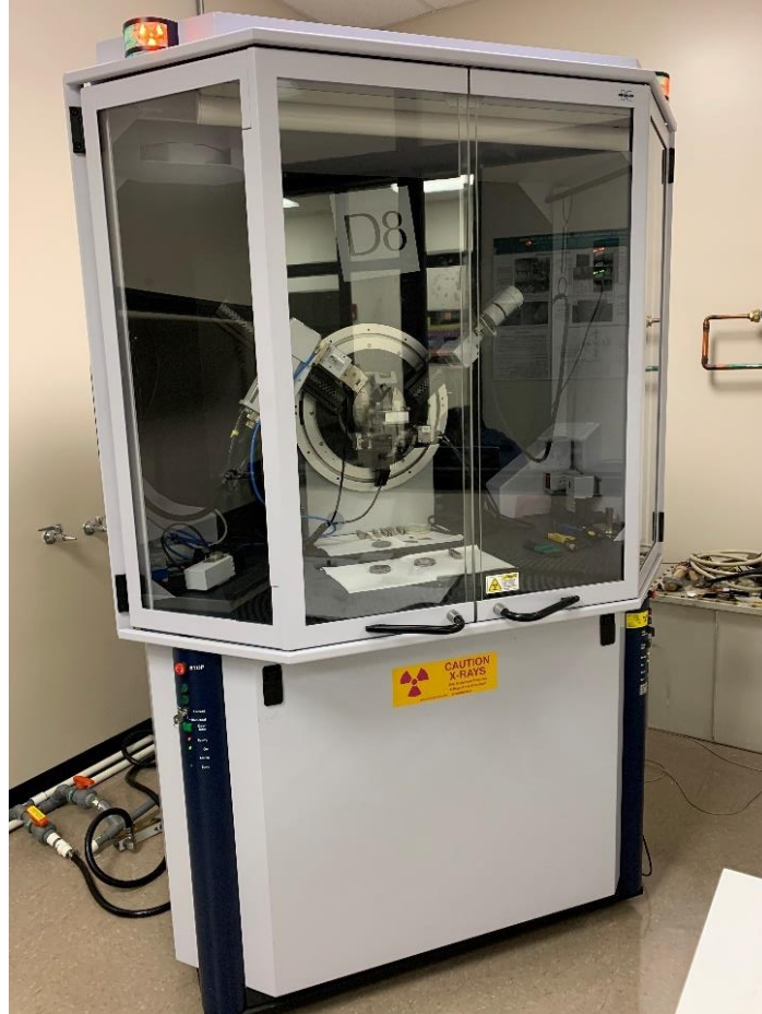
Figure 16. Bruker D8 Advance X- ray diffractometer in CCMB Lab at UTA.
