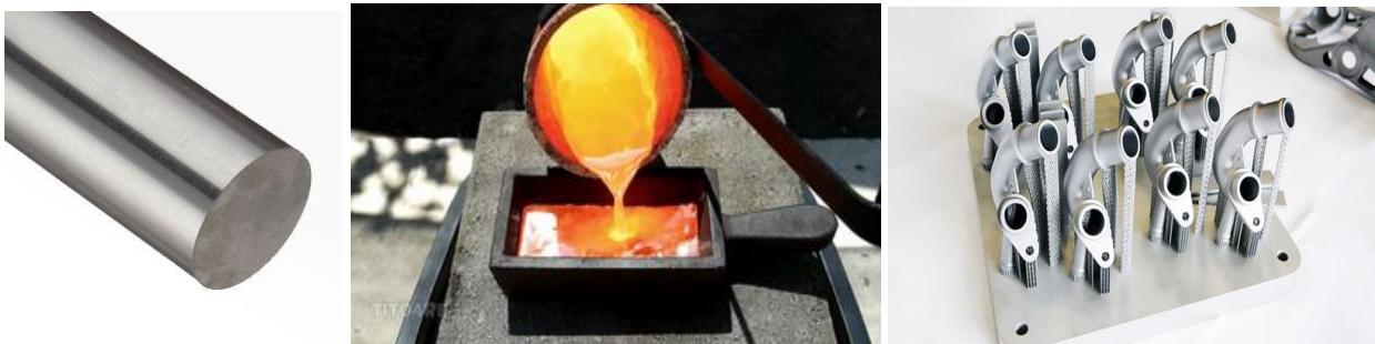
Figure 10. Inconel 718 Round Bar [134] (left), casting, and powder (middle) and water connector of an Audi W12 engine [135] (right).
