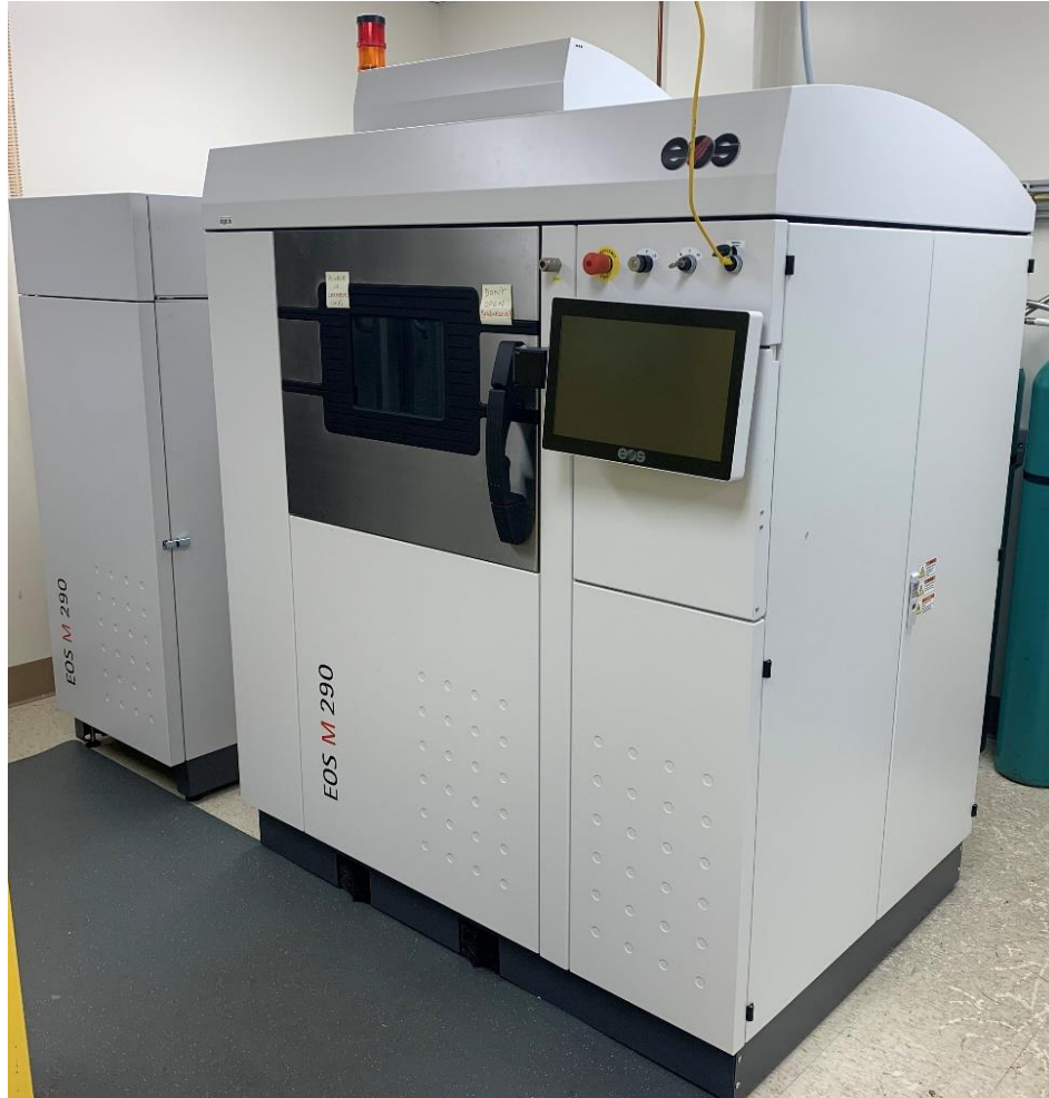
Figure 12. EOS M290 metal 3D printer with a fiber 400 W laser in UTA in IAM-Lab.
