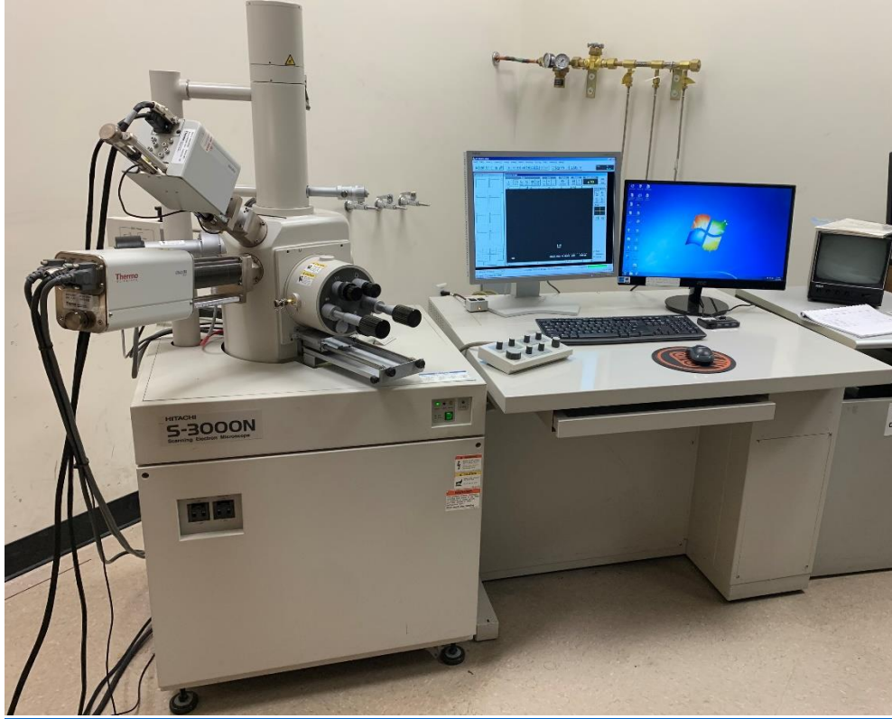
Figure 15. Hitachi S-3000N Scanning Electron Microscope in CCMB Lab at UTA.
