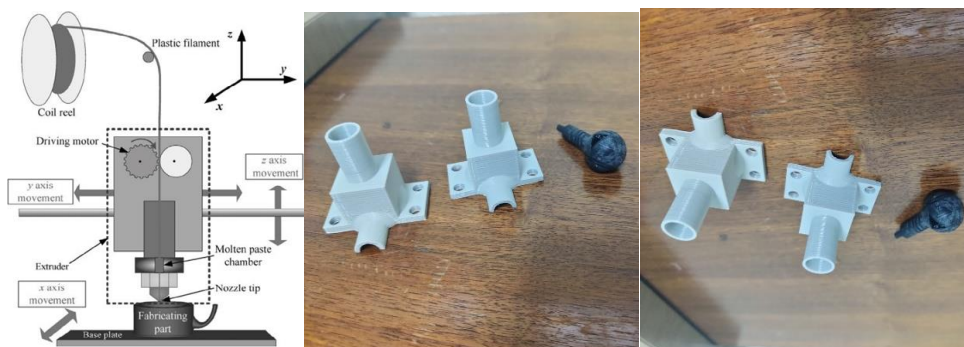
Figure 10. Schematic of FDM machine and FCD parts produced using FDM.[44]
