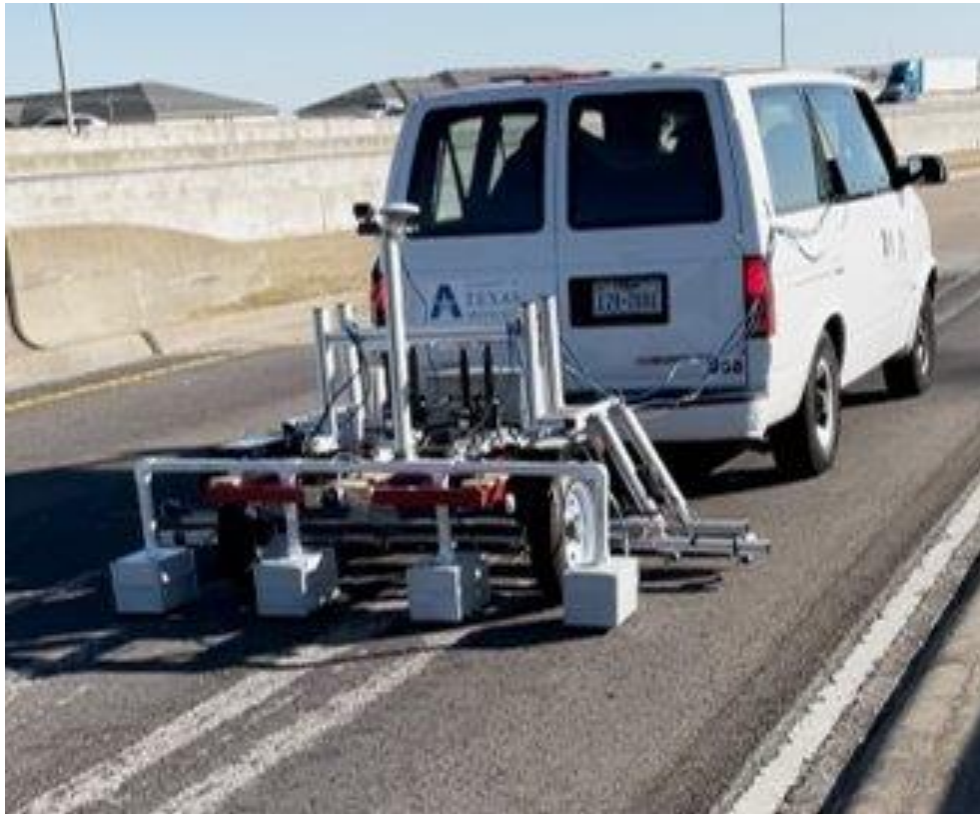
Figure 5.3. Device deployment of AHAS platform with truck and van. The device deployment allows mechanical wave, electromagnetic wave, video image, position data collection simultaneously.
