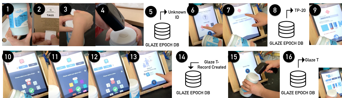
Figure 5.4: Updating inventory with newly purchased glaze: 1-4) A user is creating an entry for a newly purchased commercial glaze. She grabs an unassigned RFID tag from the dispenser and places it on the lid of the bottle. 5-8) She scans the tag and follows the prompts on the Glaze Epoch UI to assign a glaze by searching for the record from our glaze database. 9-14) She creates a unique icon for the glaze by choosing a shape, color, and a letter. 15-16) The information is stored in the database (see Video Appendix B.2).
