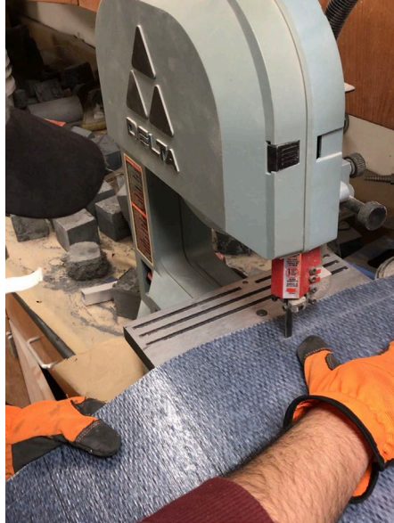
Figure 3-4 Cutting the CFRP laminate into strips (coupons)
