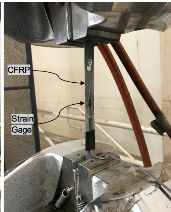
(c) CFRP specimen before conducting the tensile test
