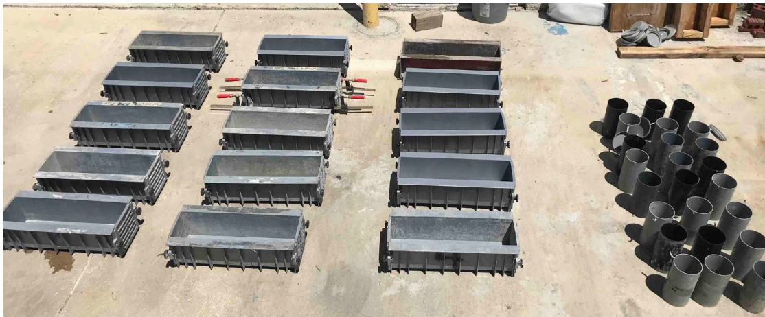
Figure 3-10 Rectangular beam and cylinder molds before casting
