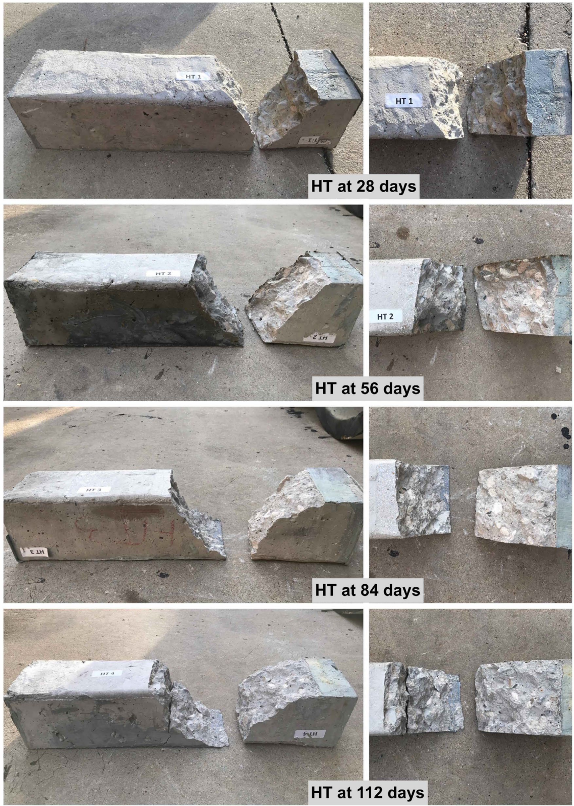
Figure C-3 Failure modes from flexural tests of specimens immersed in moderate temperature (60 °C) water for different durations
