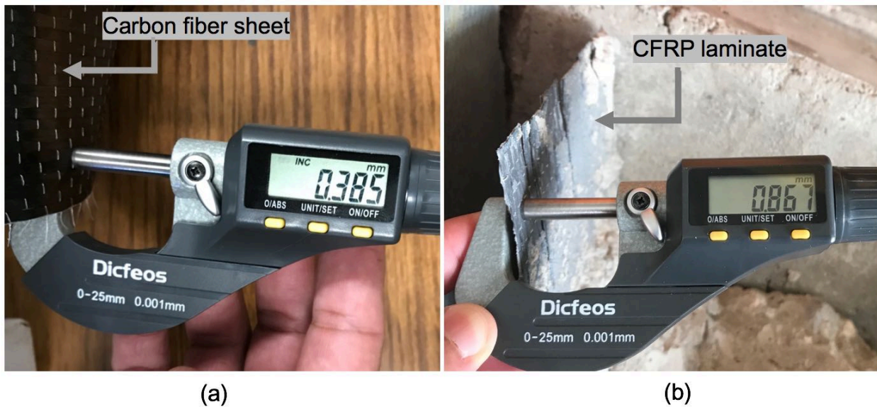
Figure 5-11 Thickness measurement: (a) measure the carbon fiber sheet, (b) measure the CFRP laminate after failure
