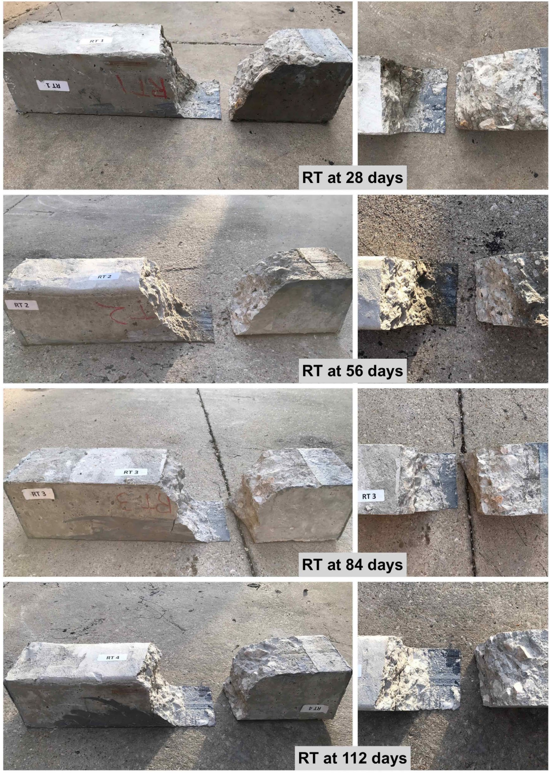
Figure C-1 Failure modes from flexural tests of specimens immersed in room temperature (23 °C) water for different durations
