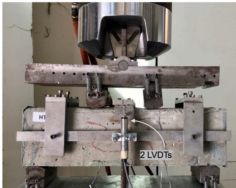
Figure 3-27 Schematic of flexural testing apparatus for three-point loading test
