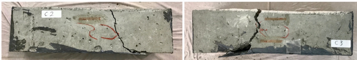
Figure 4-23 Failure modes from flexural tests of control specimens
