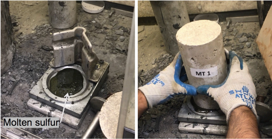
Figure 3-13 Capping of concrete cylinders
