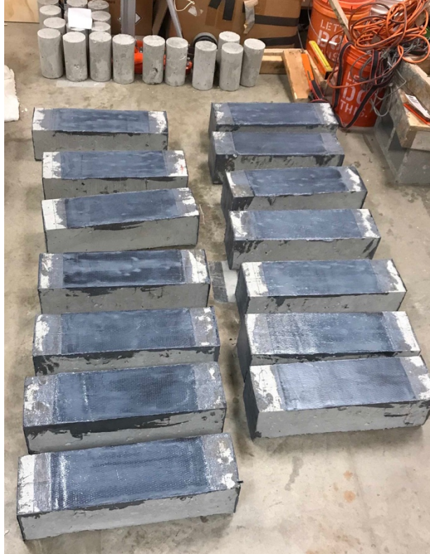
Figure 3-20 Concrete beams after applying the CFRP
