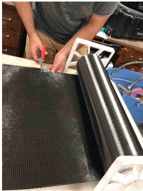
Figure 3-17 Cutting the CFRP fiber sheet
