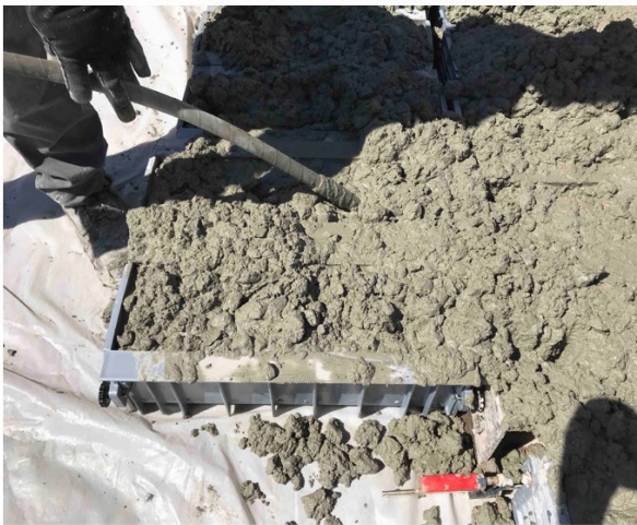
(c) using the vibrator in each mold
