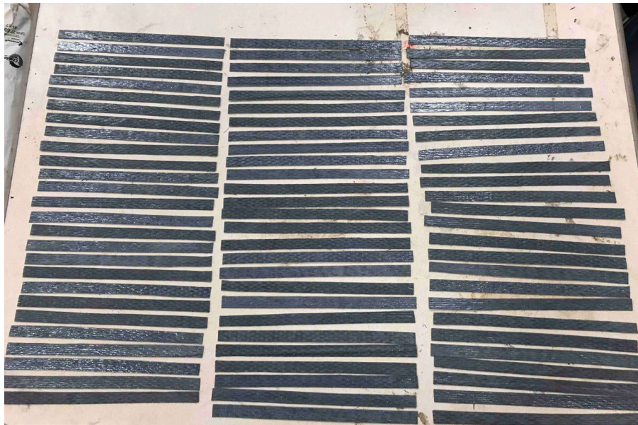
Figure 3-5 Specimens of CFRP laminate (coupons)
