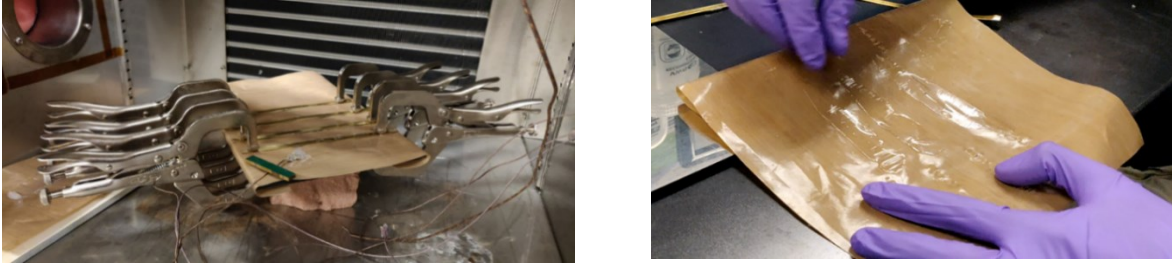
Figure 5-3: Sample preparation without the top plate (left) and cured sample (right).
