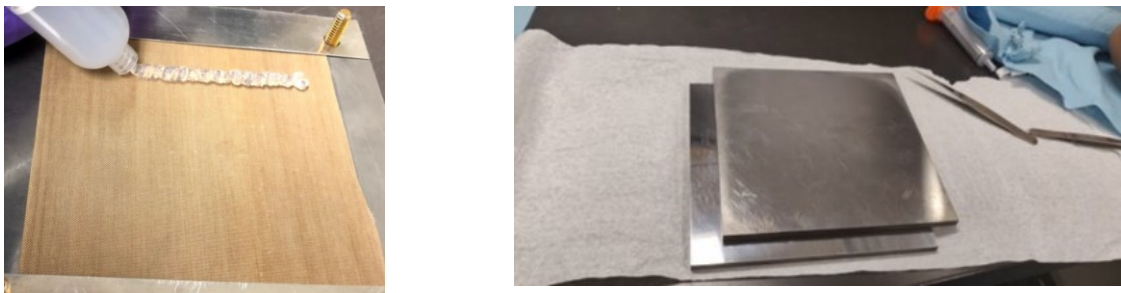
Figure 5-4: Sample dispensed on the Teflon sheet attached to the steel plate (left), assembly ready to cure on (right).
