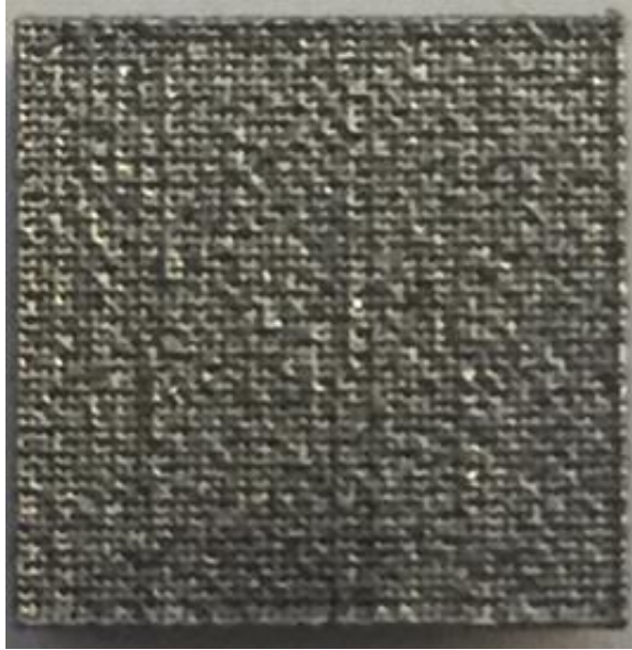
Figure 45: 3D printed surface with high roughness to increase the efficiency
