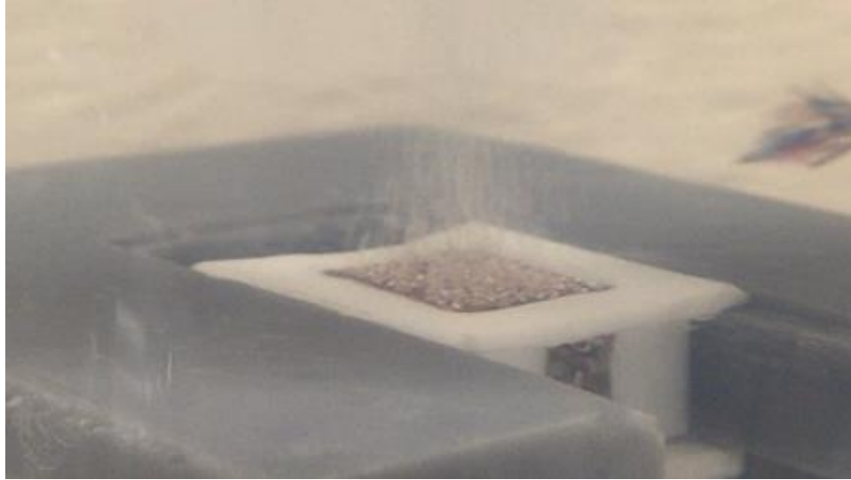
Figure 40: bubble generation on the plane surface for the power density ( 10 \text{ W/cm}^2 )
