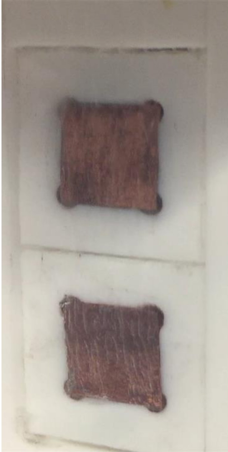
Figure 41: bubble generation on the vertical configuration of the plane surface for the power density 4 \text{ W/cm}^2
