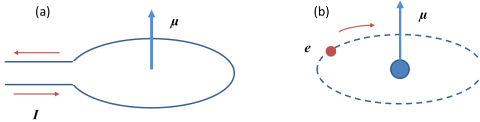
Figure 1.1 (a) The moment of a loop of wire carrying a current and (b) the moment of an electron in a hydrogen atom.
