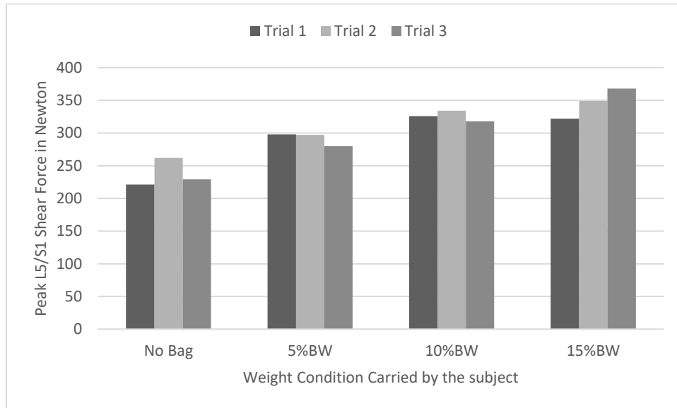
Figure 12 : Peak shear forces at L5/S1 disc (from heel strike to toe off) while walking under varying weight carrying conditions (no tool bag, 5%, 10% and 15% of BW) over three trials.
