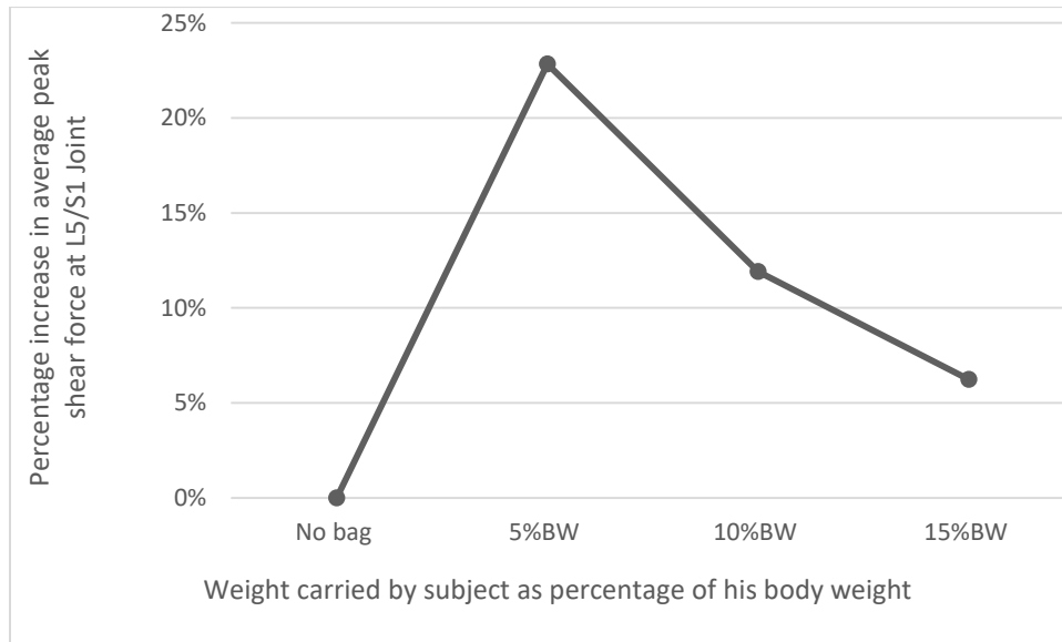
Figure 13: Percentage increase in Average Peak Shear force at L5/S1 as the weight carried by the participant increased
