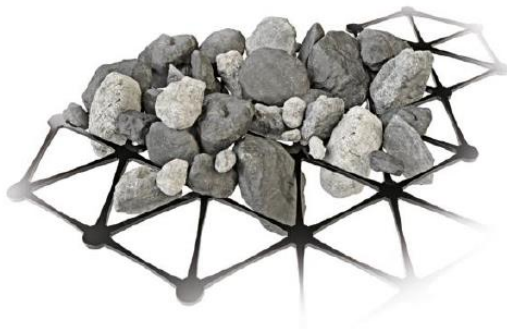
Figure 2.24: Interlocking mechanism of stiff geogrid providing lateral confinement and stabilization (Dobie et al. 2018)
