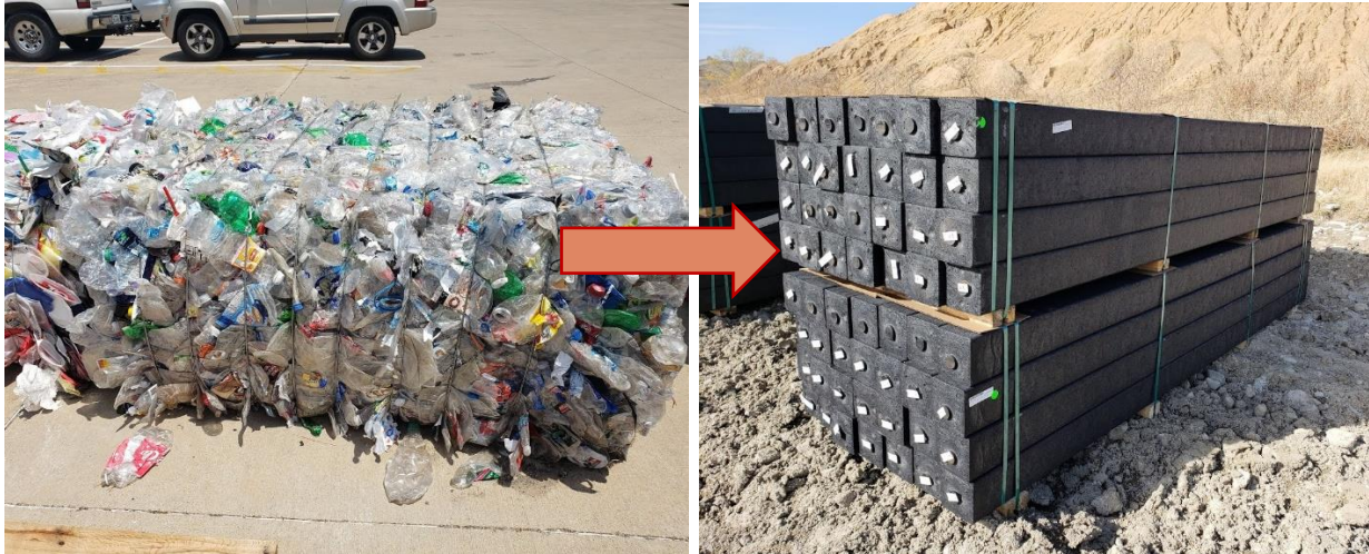
Figure 2.30: Approximately 600 plastic soda bottles are used for one 4"×4" RPP
