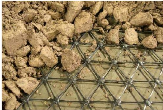
Figure 2.24: Interlocking mechanism of stiff geogrid providing lateral confinement and stabilization (Dobie et al. 2018)
