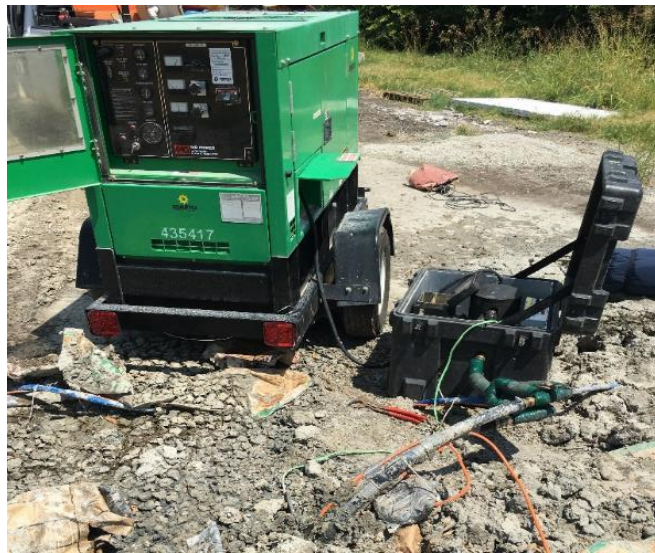
Figure 5.8. Thermal response test apparatus at the site
