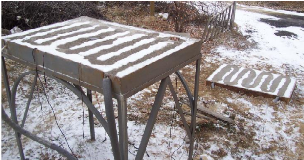
Figure 2.6. First geothermal snow-melting study in Turkey (Balbay et al. 2010)
