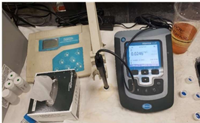
Figure 2-5: Fluoride Intellical F121 electrode probe coupled to a Hach HQ 440D base.
