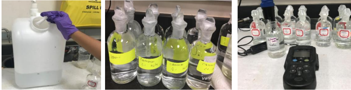
Fig 3.12 BOD reagent preparation and 0th Day and 5th Day BOD determination
