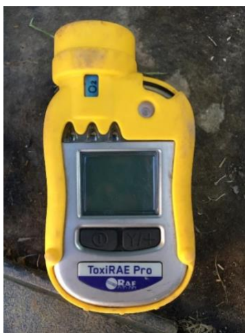
Fig 3.5 ToxiRAE Pro Oxygen sensor
