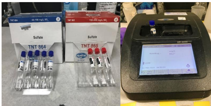
Fig 3.11 HACH 10227 method for sulfate determination
