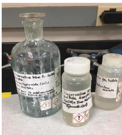
Fig 3.9 Prepared Preservative for sulfide sample preservation
