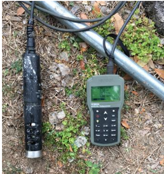
Fig 3.7 Hanna Multiparameter probe HI7698194 with the Meter HI98194
