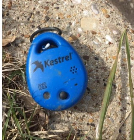
Fig 3.4 Kestrel Drop for Temperature and Relative humidity measurement
