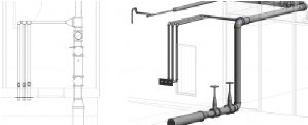
Figure 15.10 Common pipe accessories added to the fire protection system in 2D plan view (left) and 3D view (right)
