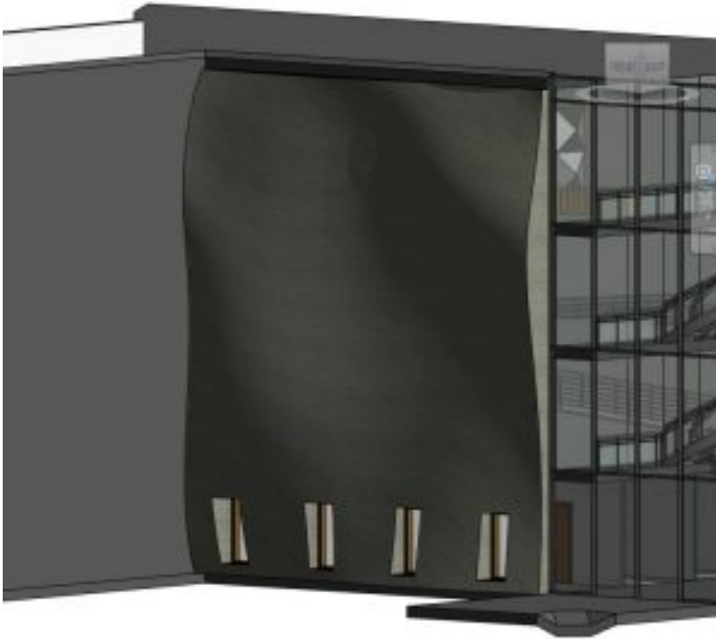
Figure 7.19 Completed Curvilinear façade shown in 3D view
