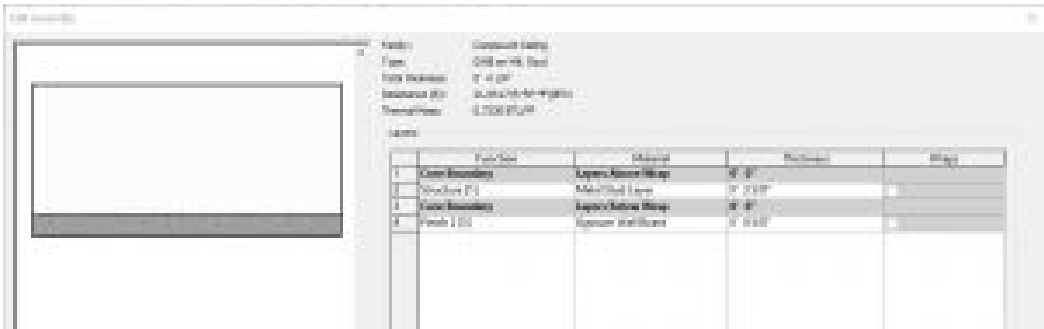
Figure 3.26 Compound Ceiling GWB on Metal Stud
