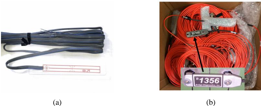
Figure 4-1 Concrete strain gage: (a) Non reusable; (b) Reusable/wireless gage
