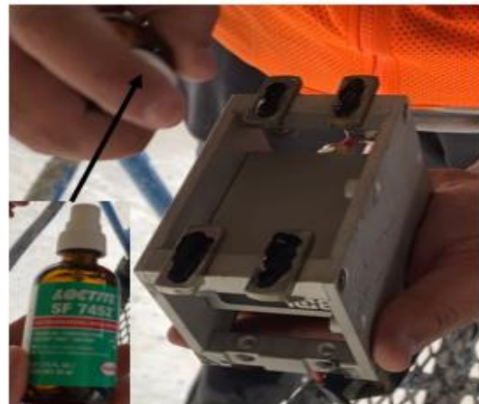
(f) Applying Loctite accelerator
