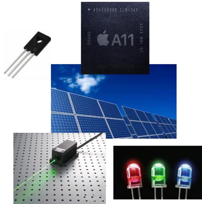
Figure 1.1: Various electronic devices created from semiconductor heterojunctions. Some examples include transistors, integrated circuits, solar cells, lasers and light-emitting diodes.
