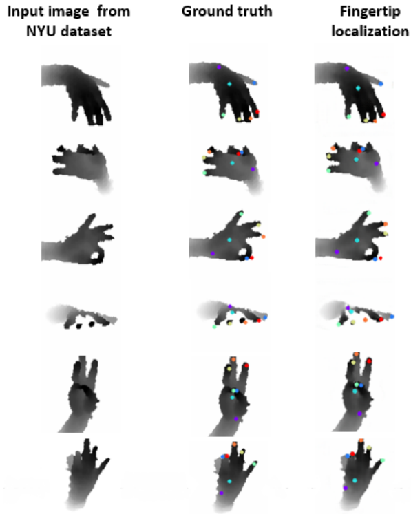
Figure 3.11. Qualitative results on examples of test data from NYU hand dataset; first column real depth image, second column ground truth locations and third column represents the translated image using Cycle-constituency approach.
