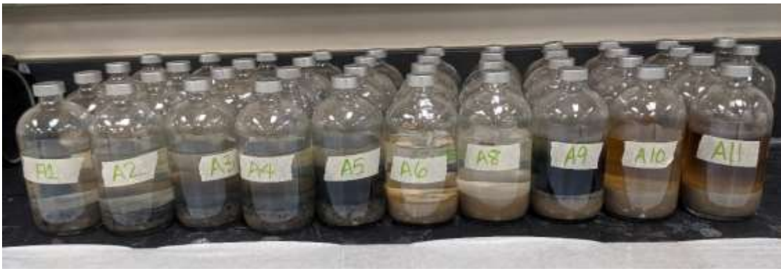
Figure 3.2. Batch experiment (soil with amendments) with synthetic leachate
