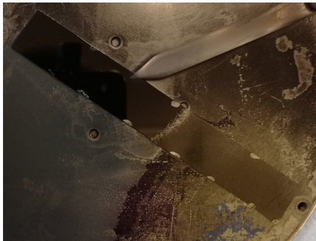
Figure 4.6: Preliminary deposition sample showing a debonded region
