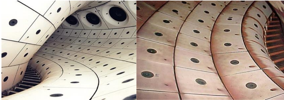
Figure 2 Optimal Failure-Finding Intervals for Heat Shields in a Gas Turbine Combustion Chamber Using a Multicriteria Approach [4]
