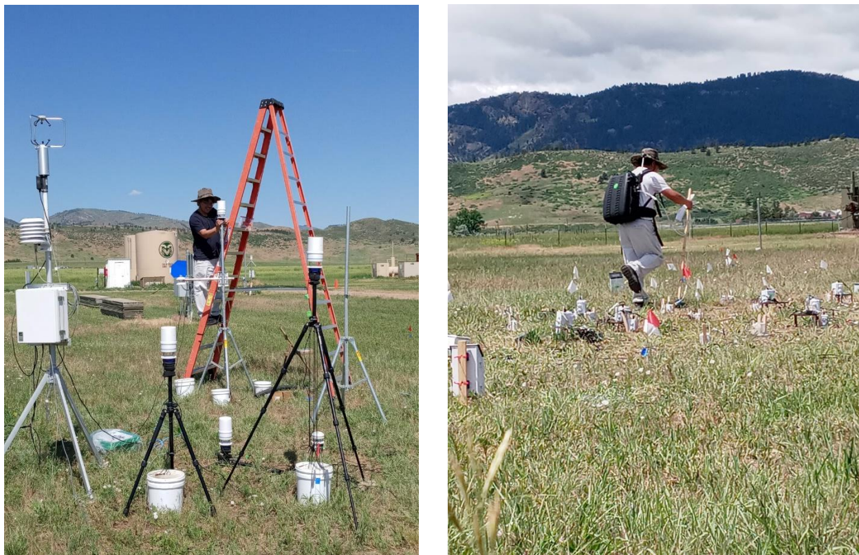
Figure A.3 Left: installments of the 3D sonic anemometer and weather sensors; Right: walking survey CH 4 measurements.
