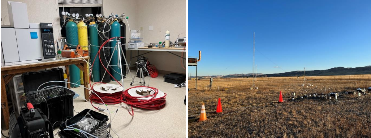
Figure A.4 Left: laboratory experiments to test the multiplexer system; Right: field 3D plume experiments using the multiplexer system.
