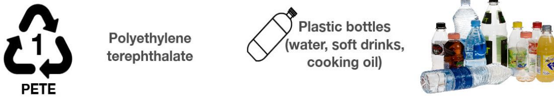
Figure 2-14 Grade 1. Polyethylene terephthalate (PET or PETE)
