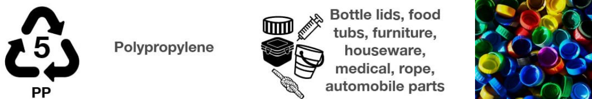
Figure 2-18 Grade 5. Polypropylene (PP)
