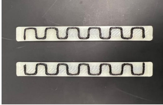
Figure 6. The 3D printed piezo-resistive strain sensor
