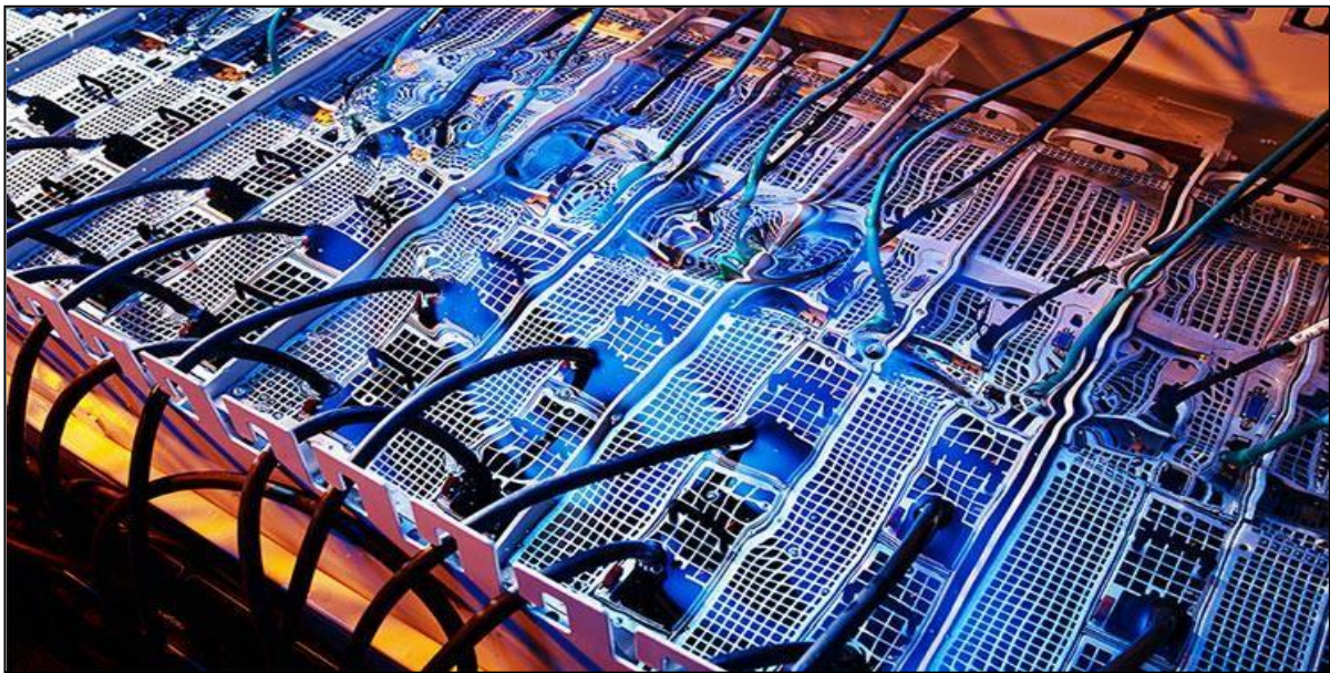
Figure 1.2 Typical Immersion Cooled Server
