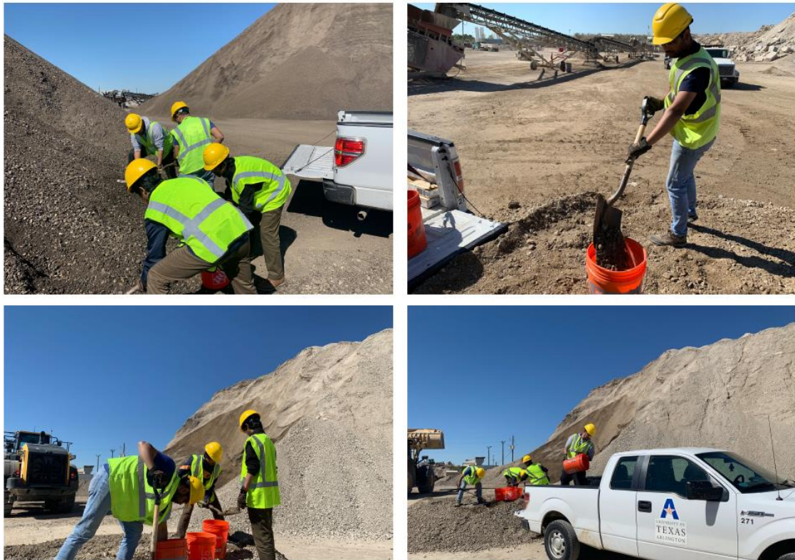
Figure 3-1 RCCA sample collection from Big City Crushed Concrete in Dallas, Texas
