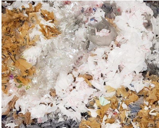
Figure 3-6 Manually shredded LDPE plastics
