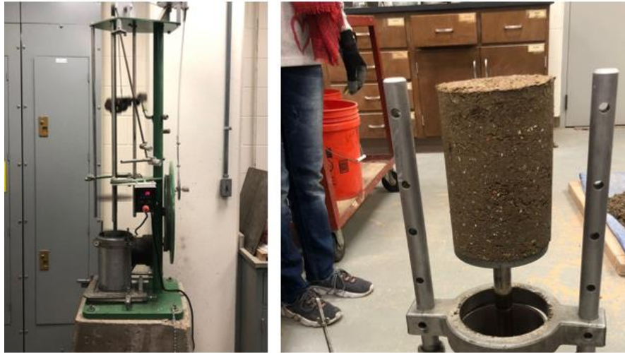
Figure 3-12 Compaction & specimen extrusion
