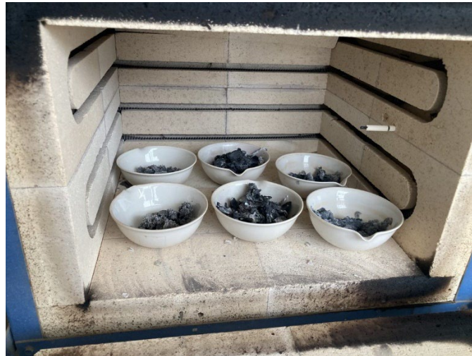
Figure 3-9: Residue or ash content of food waste after the ignition
