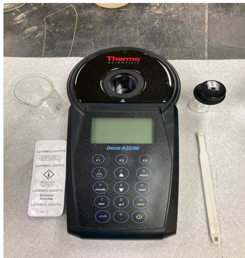
Figure 3-15: Photograph of a Colorimeter used for Alkalinity determination
