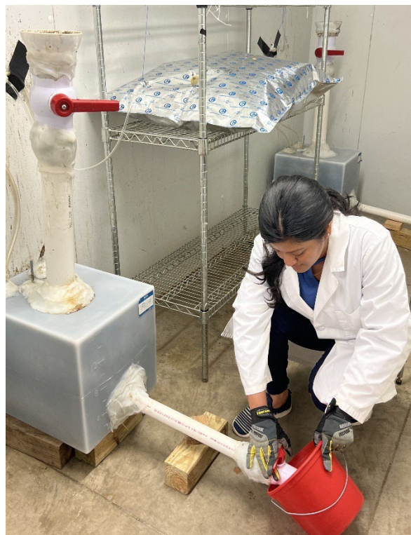
(b) Extraction procedure of the digestate
