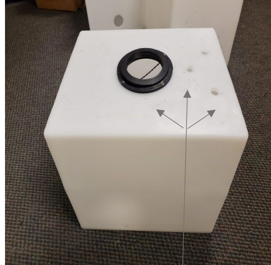
(b) Holes for the inlet, gas pipes, stirrer
