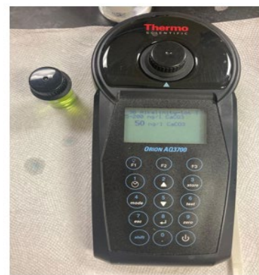
c) Measuring Alkalinity Content in mg/L CaCO 3
