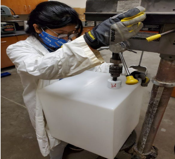
(a) Making Holes for inlets and outlets
