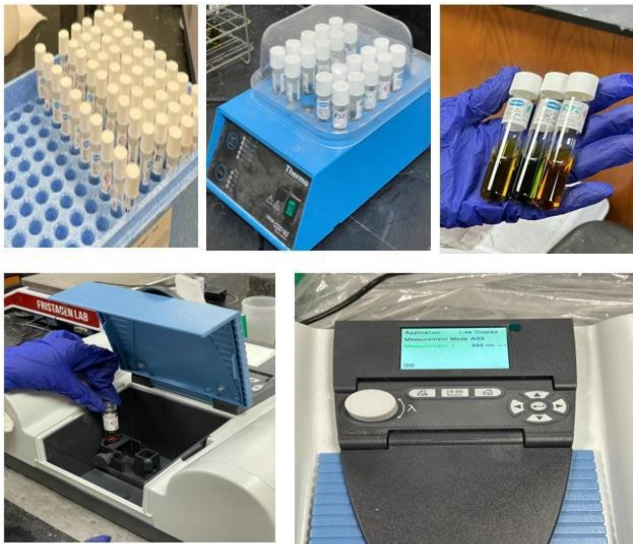
Figure 3-12: Determination of Chemical oxygen demand (COD): (a) COD vials, (b) digester heating, (c) vials after heating; (d) vials placing in Spectronic 200+, (e) measurement of absorbance by s Spectronic 200+
