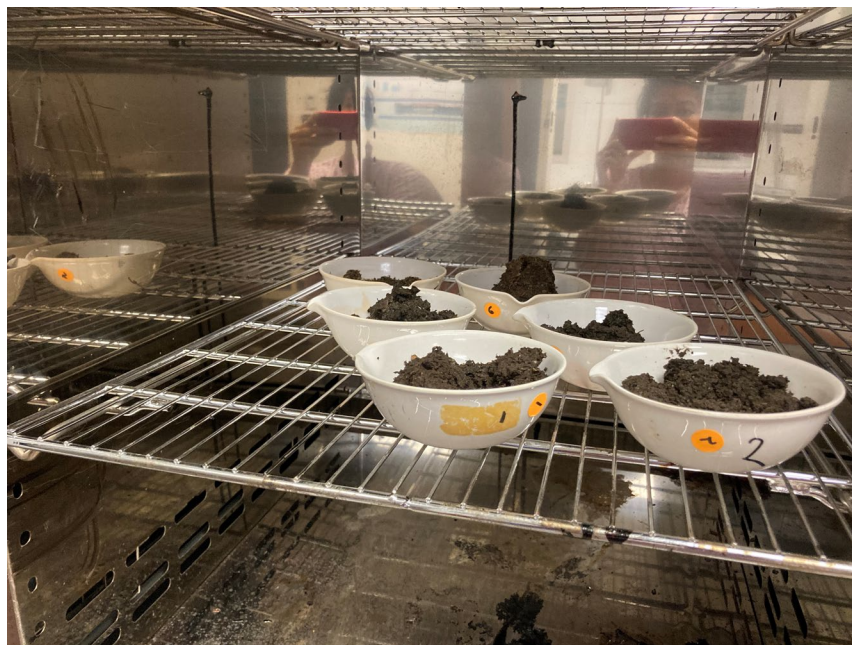
Figure 3-8: Determination of moisture content by drying sample in the oven
