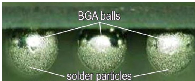
Figure 1- 6 View of BGA Solder Ball [7]
