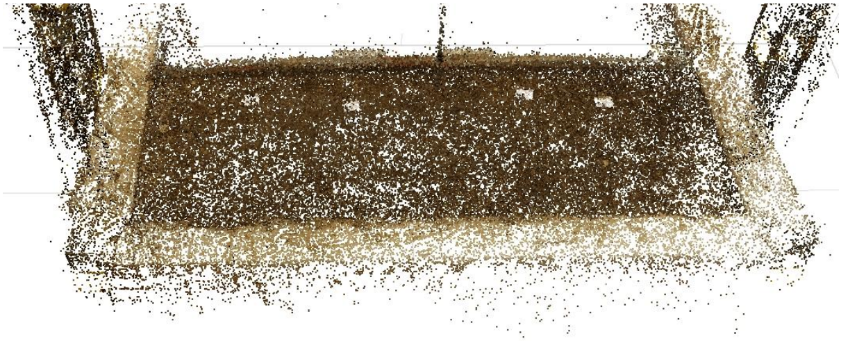
Figure 37: Sparse cloud points of the surface (before pullout test), for test 1 (embedment depth 65cm).
