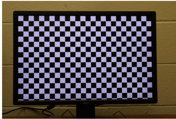
Figure 22: Chessboard generated by Metashape for camera calibration
