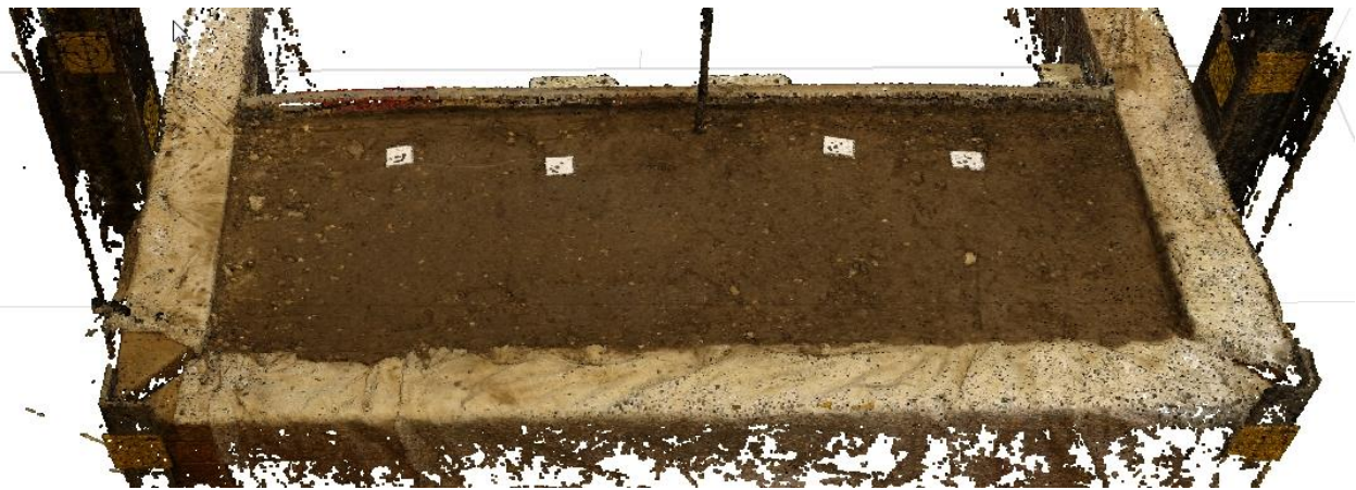
Figure 38: Dense cloud points of the surface (before pullout test), for test 1 (embedment depth 65cm).
