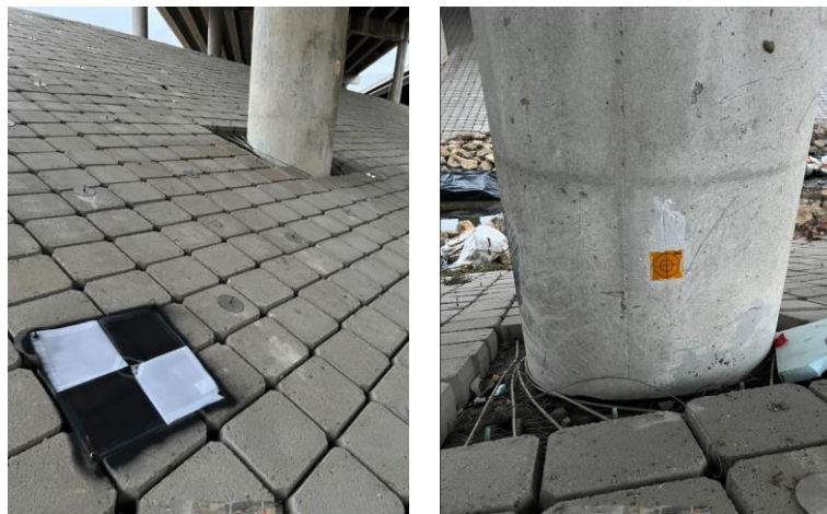
(a) (b) Figure 33: Placement of (a) GCPs and (b) Reflective targets in the site
