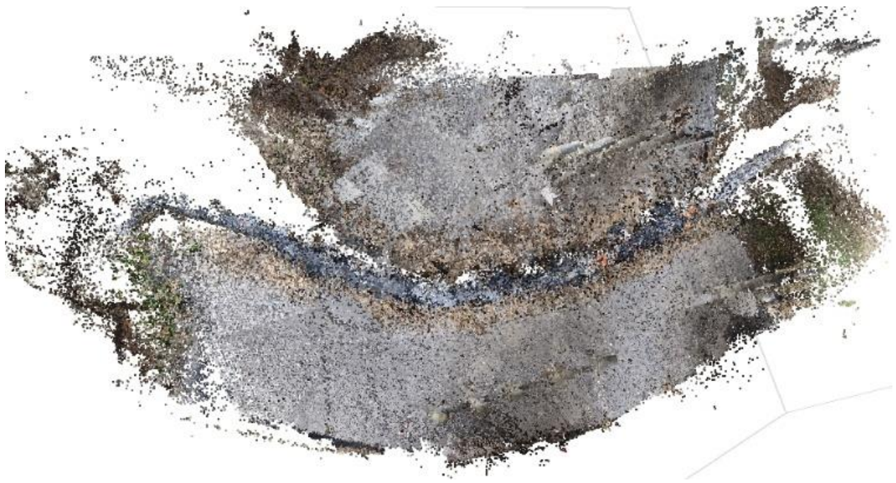
Figure 52: Unfiltered sparse cloud of slope
