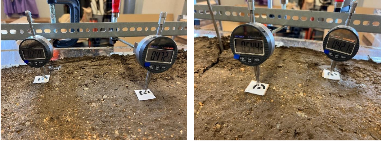
Figure 41: Dial gauge readings after the second test (point 1 on left)
