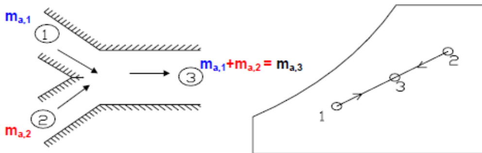
Fig 18 - Adiabatic mixing schematic with process line on the psychrometric chart [25]
