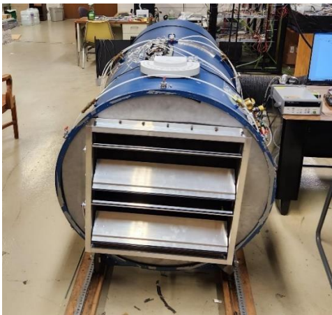
Fig 14 – Image of Front section of Air flow bench
