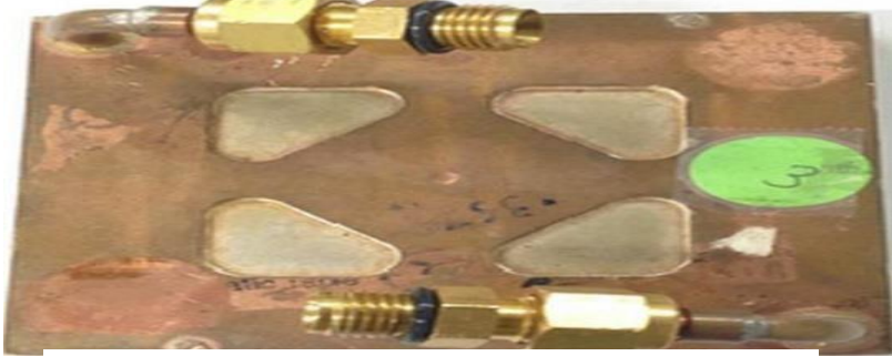
Figure 9: Cold plate used in direct to chip cooling [11]
