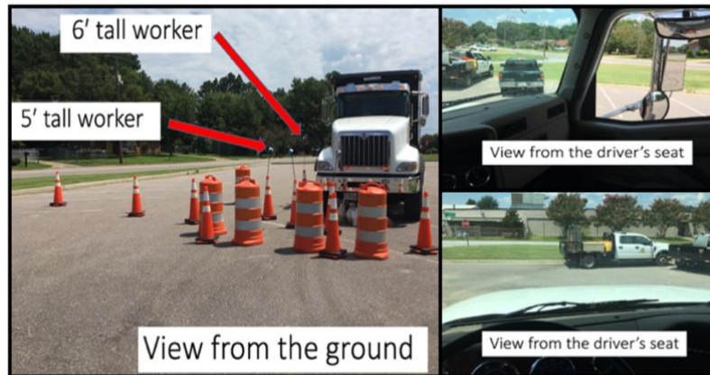
Figure 0-4. Driver's view of inspector/worker (Source: Alabama Department of Transportation Pilot Report, 2019)
