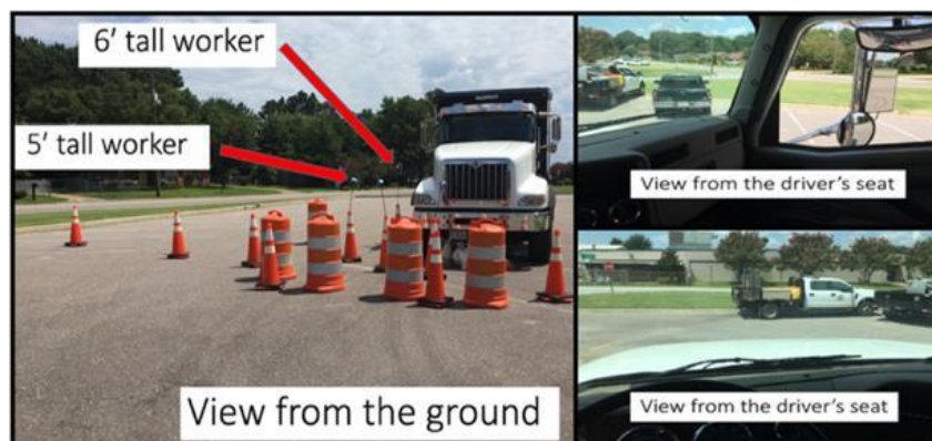
Figure 0-5. Driver’s view of inspectors/workers
