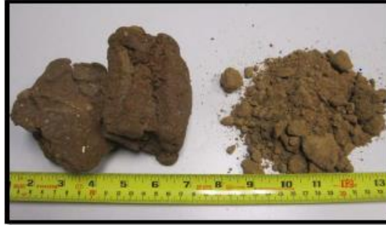
Figure 2.1 Clay soil before and after treatment with lime (TxDOT, Treatment Guidelines for Soils and Base in Pavement Structures, 2019)
