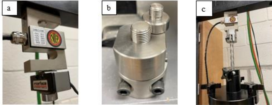
Figure 4.12 Load cell modifications for triaxial extension test: (a) Load cell interface cap for compression tests, (b) Coupler adapter for extension test, (c) Coupler adapter secured to the load cell (c)
