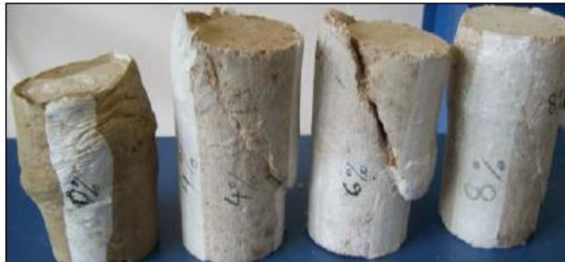
Figure 2.12 Triaxial compression (CU) samples after the test (Lucian, 2013)
