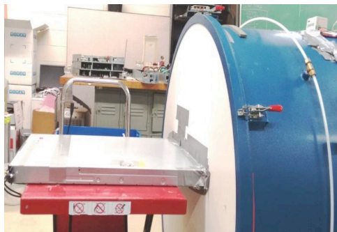
Figure 14: HP SE1102 1-RU server mounted on the airflow bench
