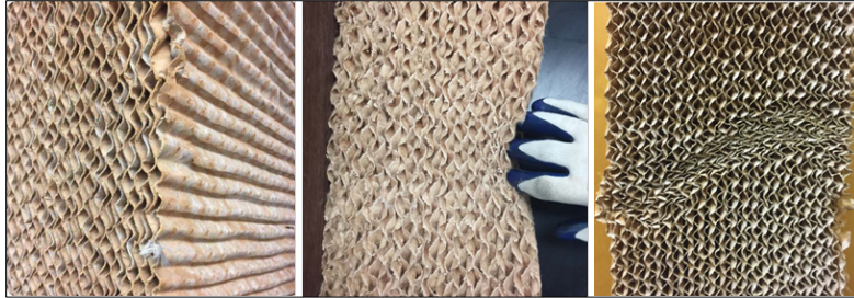
Figure 1: Scale formation, softening and collapsing of media pad (Left to Right)
