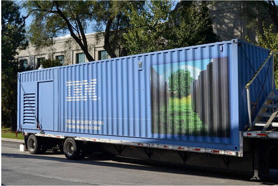
Figure 2: An IBM Modular Data Center [3]
