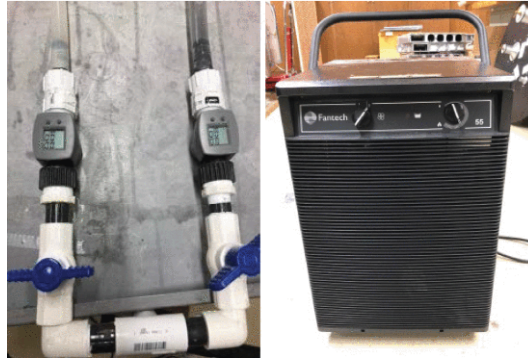
Figure 5: Digital water flow meter on each water supply and Fantech Dehumidifier
