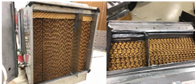
Figure 8: Side and Top view of the DEC pad fitted inside the middle duct
