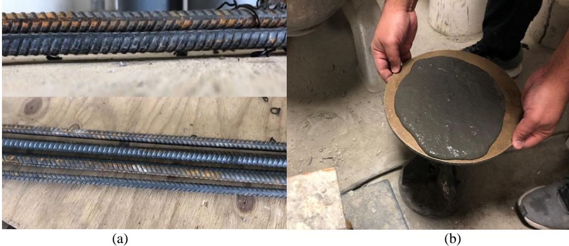
Figure 3-4 a) congested reinforcement with two layers of steel rebars and b) the high-workability of UHP-FRC
