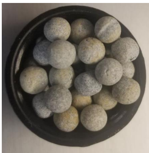
Figure 58. Thermally modified SC-MAM catalyst support prior to impregnation.
