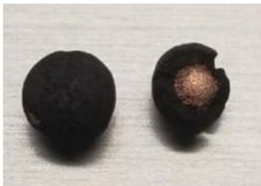
Figure 49. Core-Shell catalyst support with 2 mm copper core coated with impregnated MAM shell.
