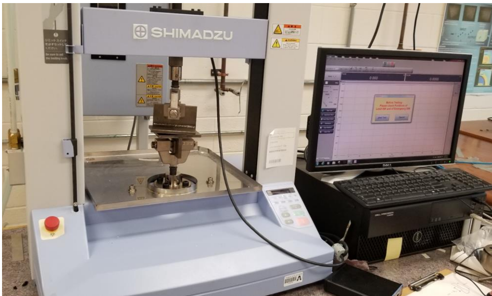
Figure 44. The lay out of the Shimadzu Precision Universal - tensile/crush tester (TCE-N300).
