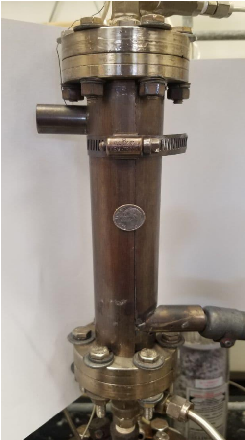
Figure 28. Actual FT reactor demonstrating the 1.9 cm reactor tube surrounded by a 4.5 cm diameter stainless steel shroud with an entry and outlet maintaining hot air flow to keep the wall of the reactor in a desired temperature.
