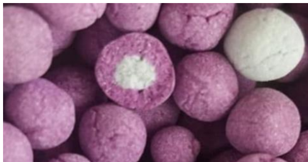
Figure 52. Egg-shell impregnated thermally modified Al-MAM support prior to calcination.
