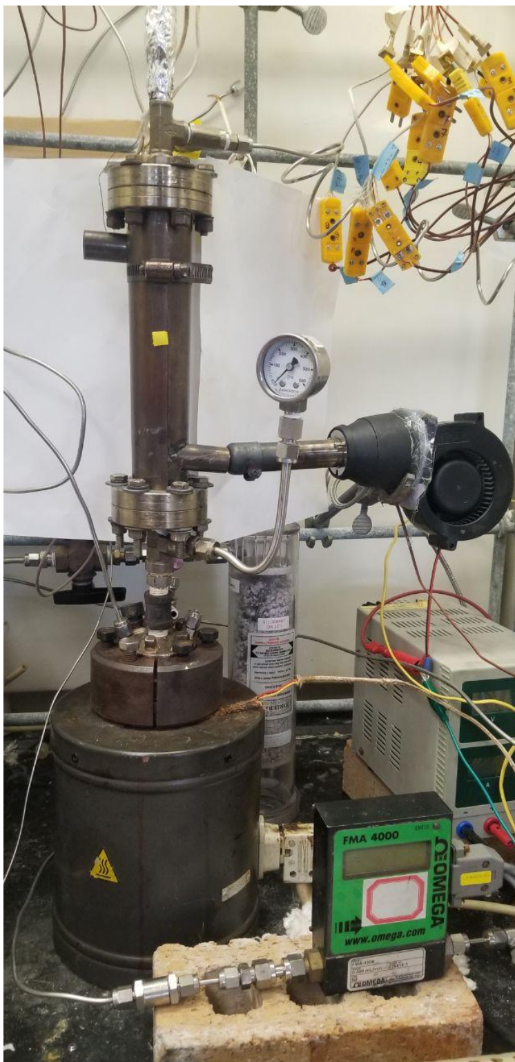
Figure 36. The Fischer-Tropsch Reactor with multi-point thermometers on top and a hot trap sample collector at the bottom.
