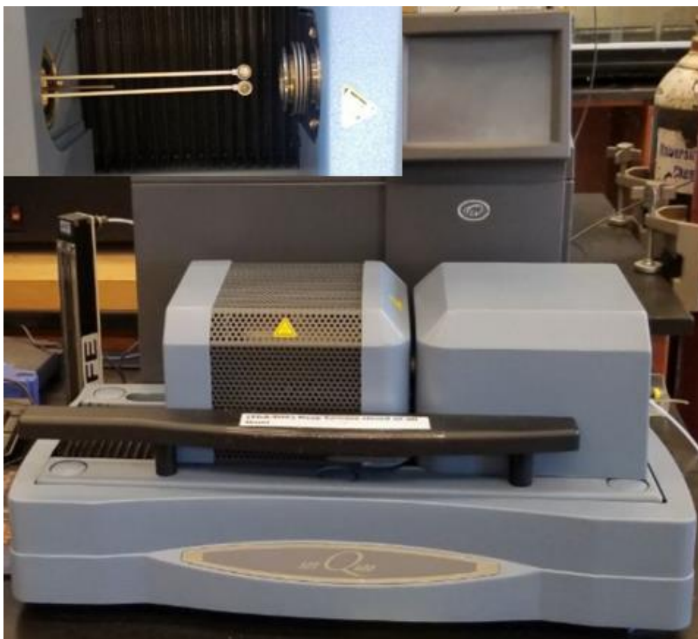
Figure 42. TPR experiments carried out via TA Instruments, the Q600 DSC-TGA with dual beam sampler and reference,
