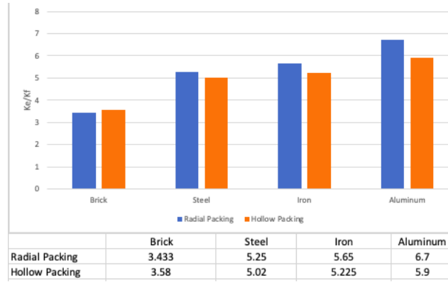
Figure 6.16: Highest ETC comparison for radial and hollow packing with aspect ratio of 8.2
