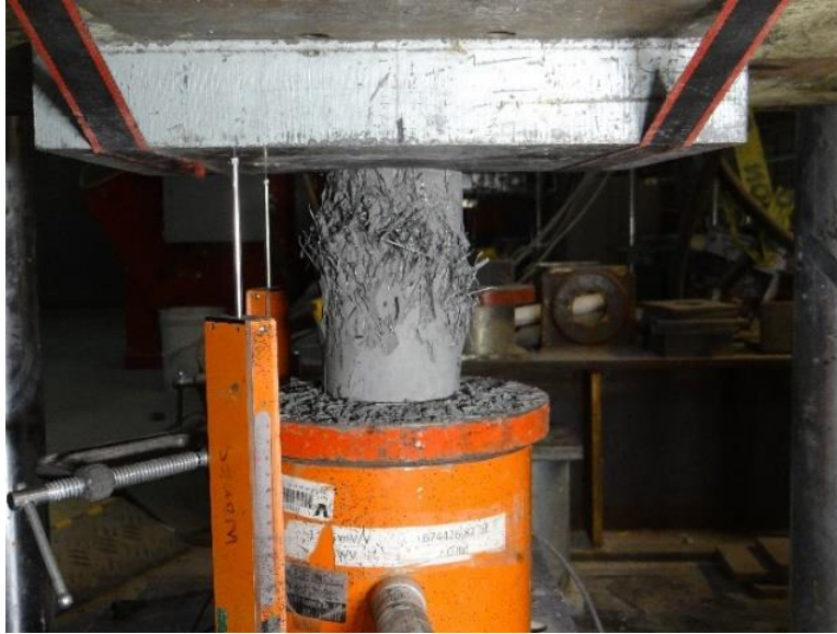
Figure 3.48 Typical Bulging-Like Failure of SIFCON (10% V_f )
