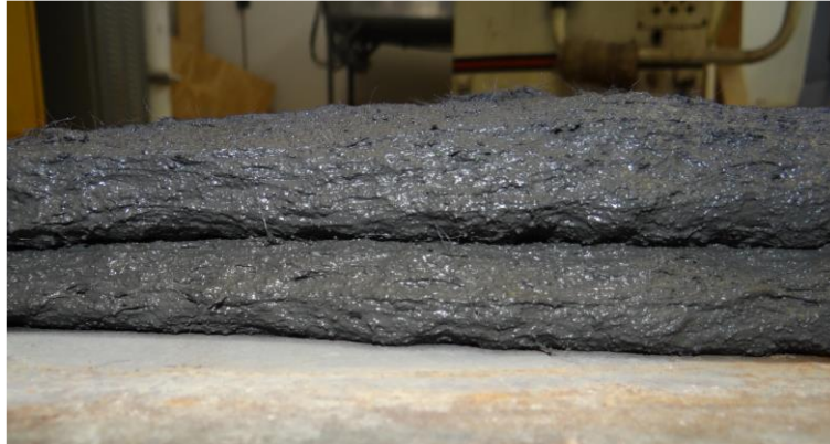
Figure 3.7 Double Layers (3D Printed UHP-FRC)
