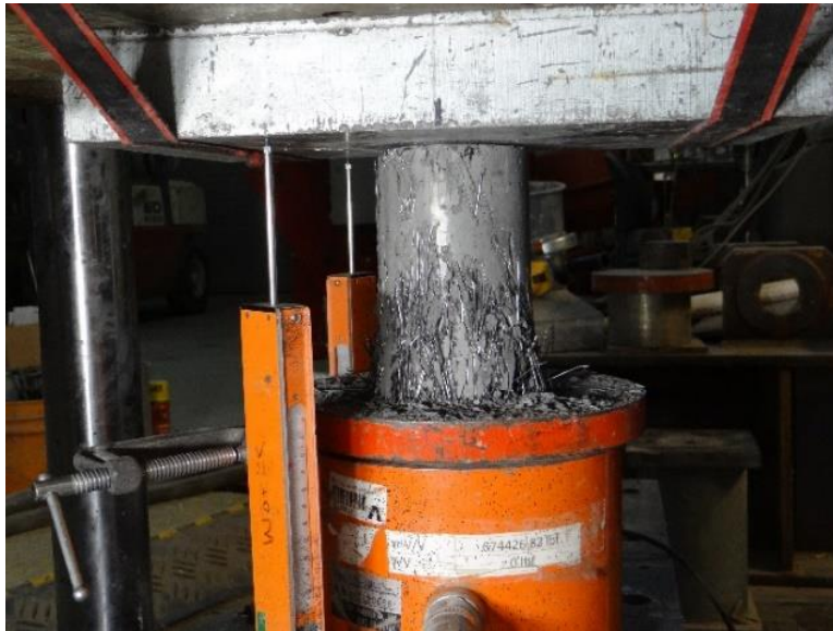
Figure 3.47 Typical Bulging-Like Failure of SIFCON (fiber type A, 10% Vf)
