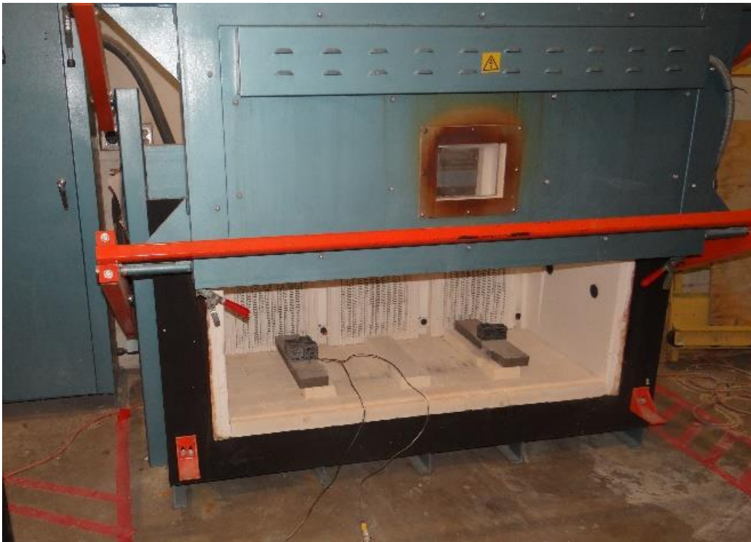
Figure 3.108 UHP-FRC cubes inside the furnace, ready for heat application
