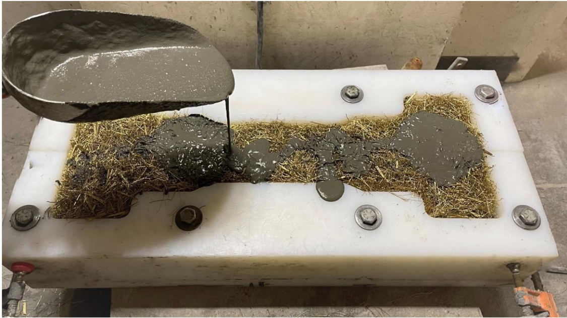
Figure 3.36 Dog Bone Shaped Specimen (filled with steel fibers, infiltration of concrete)
