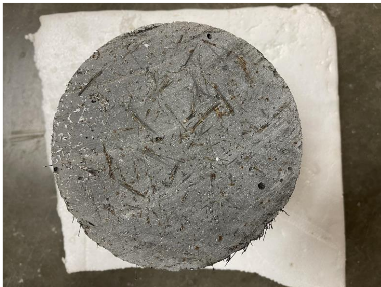
Figure 3.43 SIFCON Cylinder after Cutting the Top (fiber type A)
