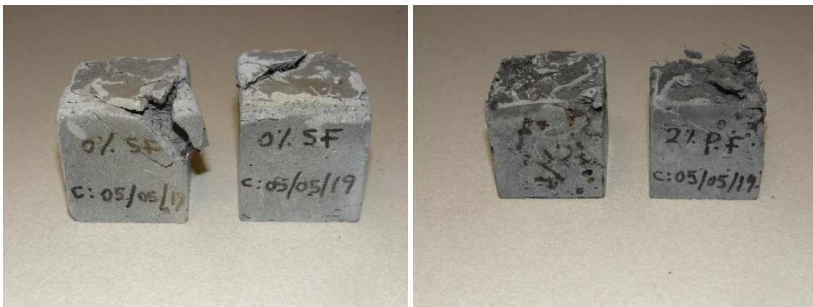
Figure 3.115 Spalling of UHP-FRC (a) without silica fume, mix 4 (b) with 2% PP fiber and 1% steel fiber, mix 5
