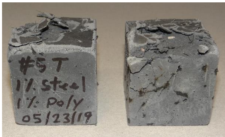
Figure 3.118 Spalling of UHP-FRC, mix 10
