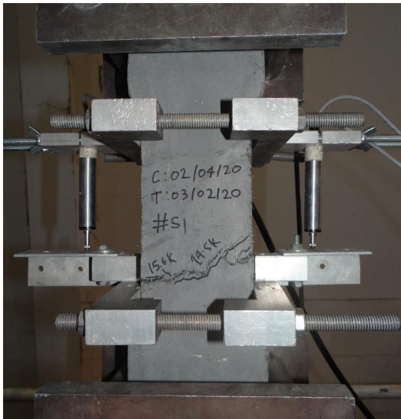
Figure 3.94 Dog Bone Specimens (smooth HiPer fiber, 3%)
