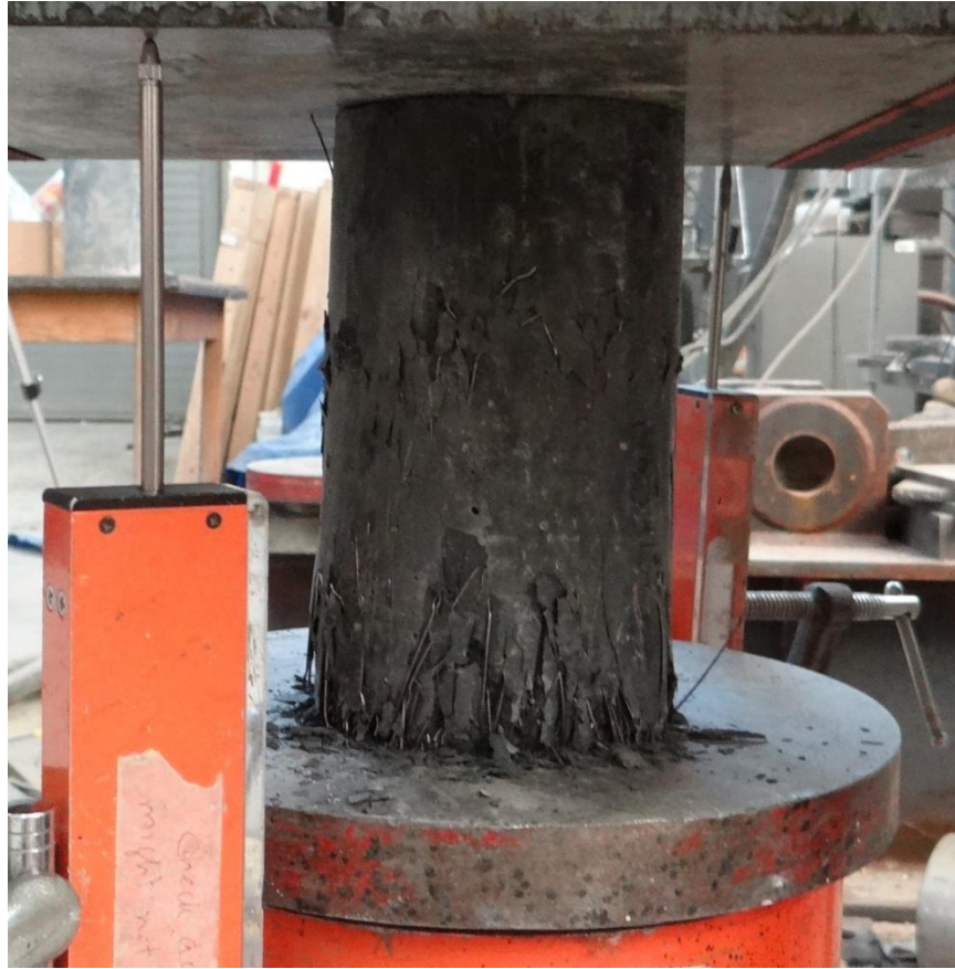
Figure 3.56 Failure Starting From the Outside Surface (Cylinder)
