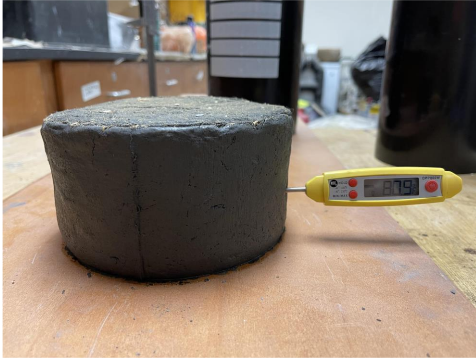
Figure 3.6 Recorded Temperature of Mix
