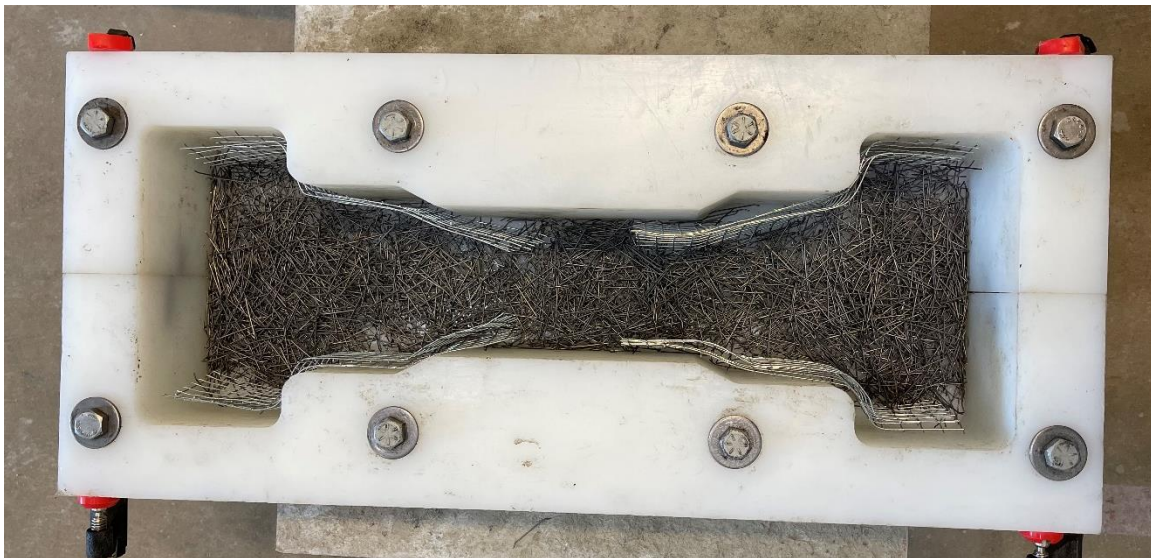
Figure 3.32 Dog Bone shaped specimen (showing side reinforcement)
