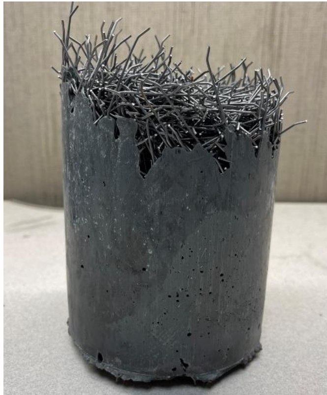
Figure 3.53 SIFCON Cylinder with Hooked-Ends Steel Fibers Half Infiltrated by UHPC Slurry
