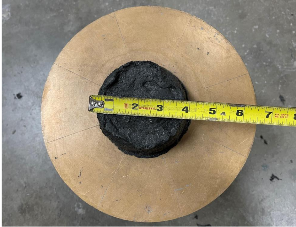
Figure 3.5 Flow Measurement of 3D Printed Mix
