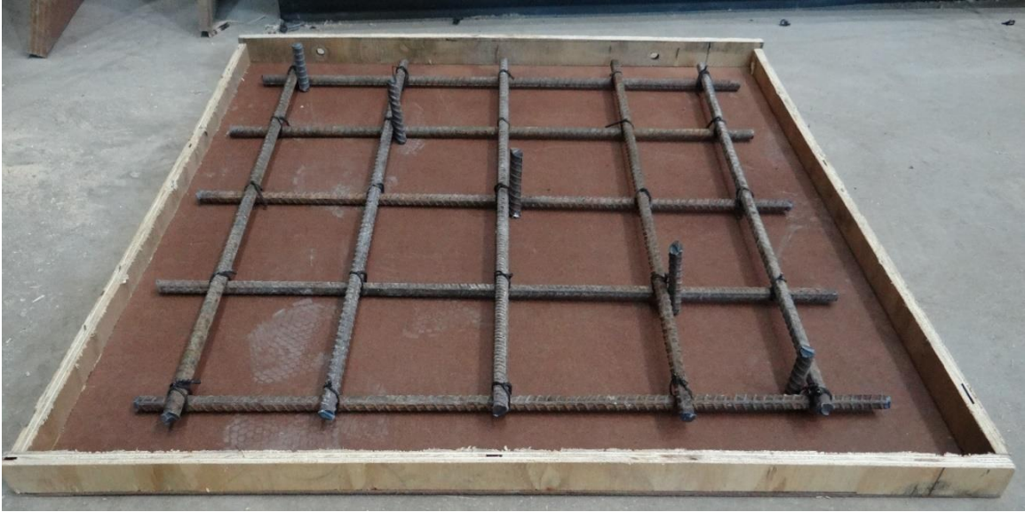
Figure 3.104 Rebar Cage for the UHP-FRC Panel
