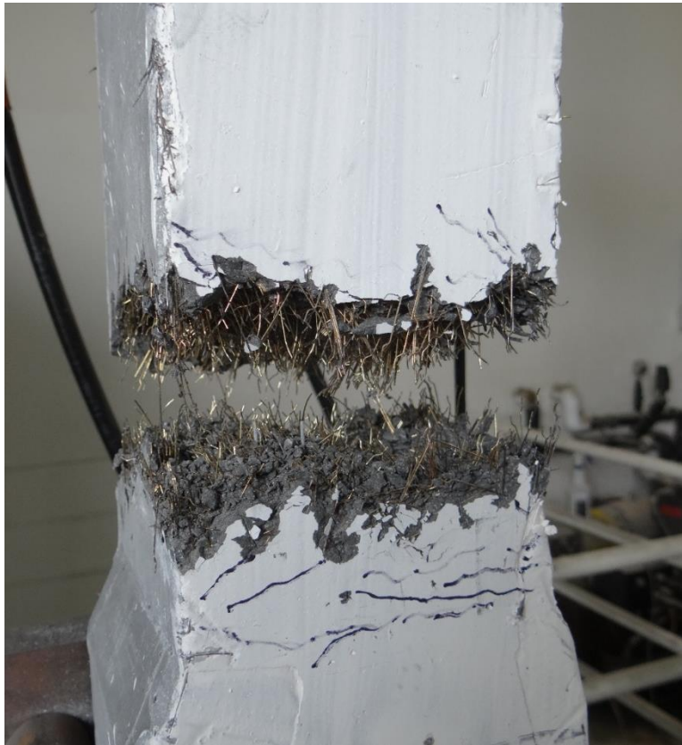
Figure 3.74 Initiation of Cracks (dog bone specimen for SIFCON, fiber type B)
