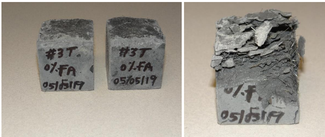
Figure 3.113 Spalling of UHP-FRC at high temperature (a) mix 1 (b) mix 2
