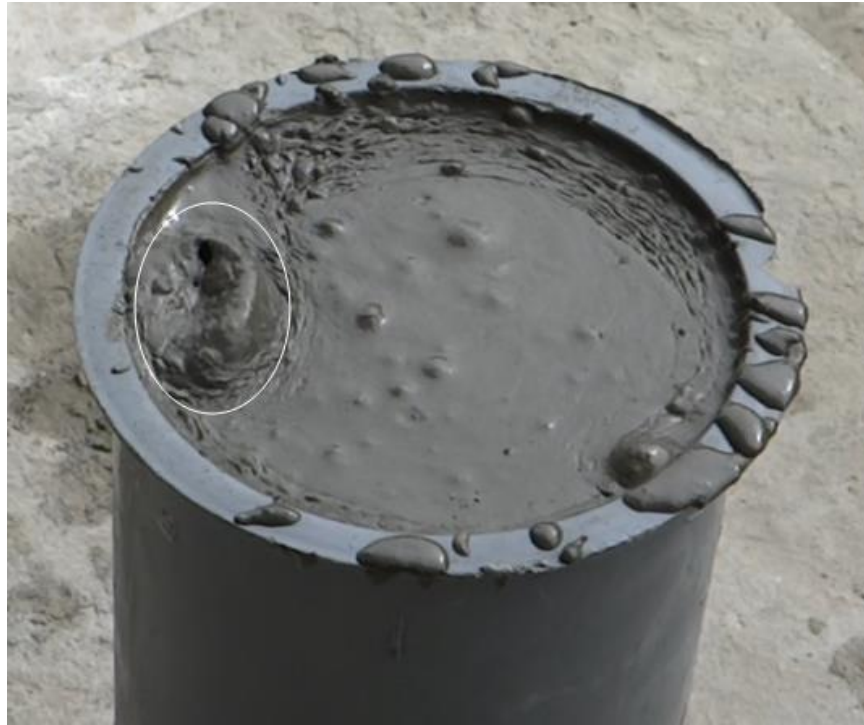
Figure 3.37 Formation of Air Voids during the Infiltration of UHPC paste
