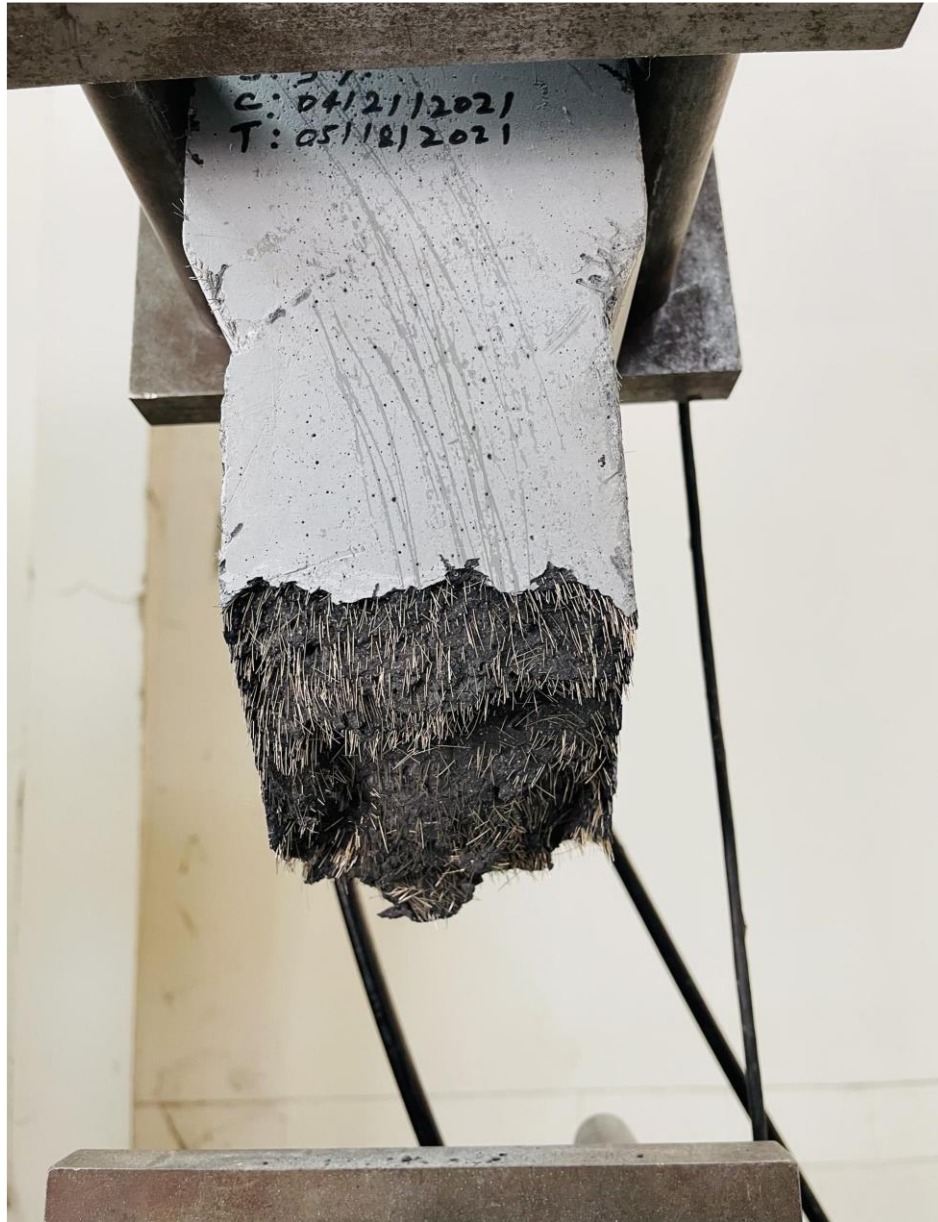
Figure 3.91 Pull-out of Fibers (Dog Bone Specimens (deformed fiber, 3%))
