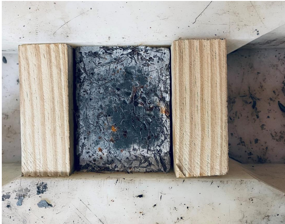
Figure 3.39 Anisotropic Behavior of SIFCON (Naaman et al., 1998)
