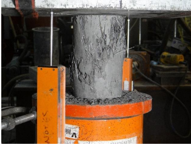
Figure 3.46 Typical Shear-Like Failure of SIFCON (fiber type A, 10% Vf)
