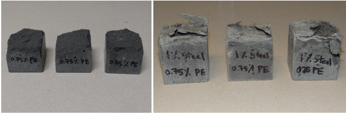
Figure 3.113 Spalling of UHP-FRC at high temperature (a) mix 1 (b) mix 2
