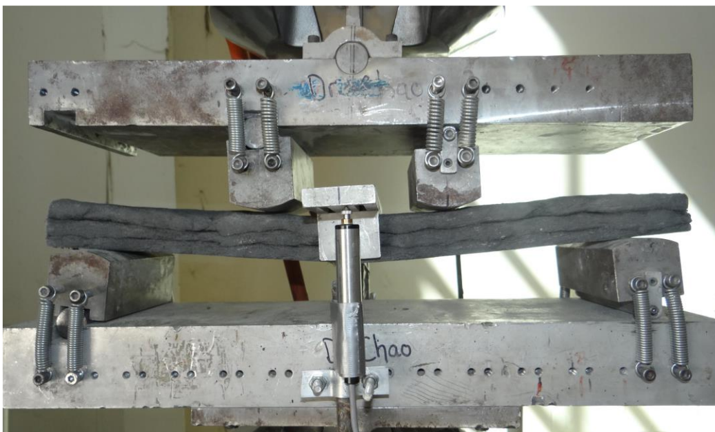
Figure 3.24 3 rd Point Bending Testing of 3D Printed Beam
