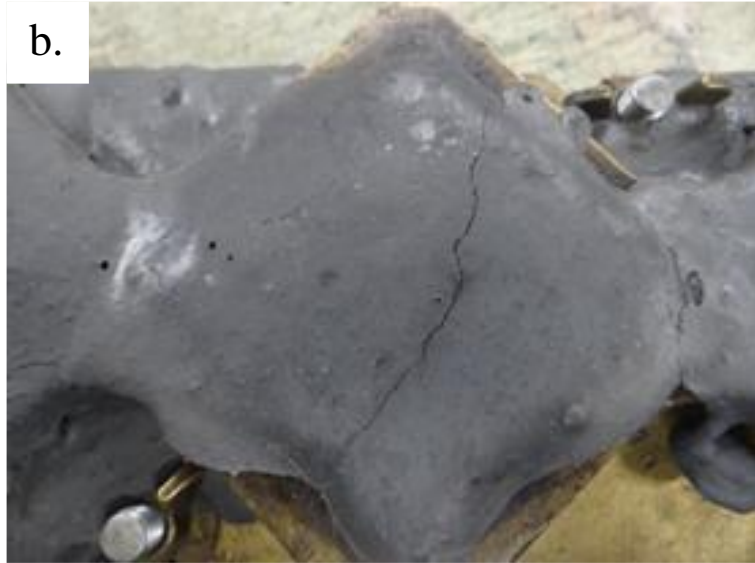
Figure 3.124 (a) Swelling of ULW- UHP-FRC (b) Cracks at the Surface of ULW- UHP-FRC
