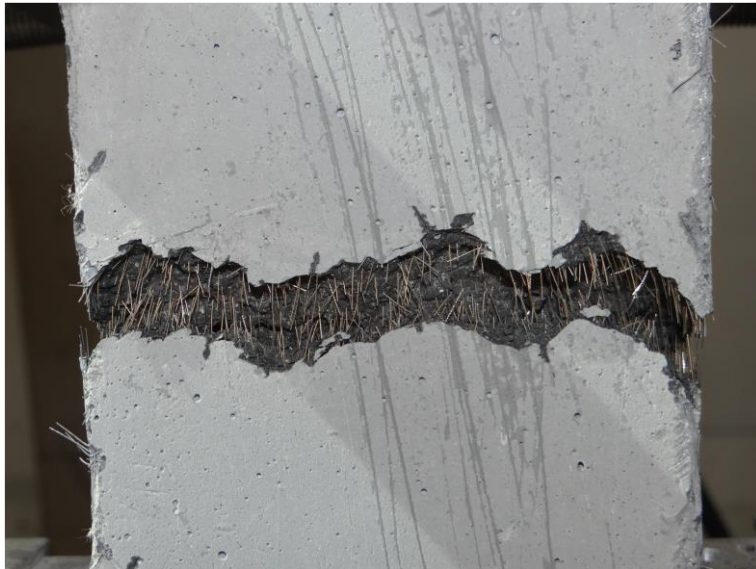
Figure 3.90 Crack Zone (Dog Bone Specimens (deformed fiber, 3%))
