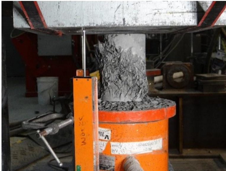
Figure 3.49 Typical Bulging-Like Failure of SIFCON Followed by Shear-Like Failure (10% V_f )
