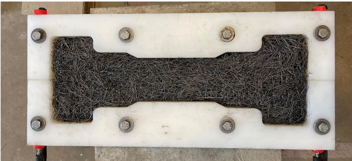
Figure 3.34 Dog Bone Shaped Specimen (filled with steel fibers, fiber type A)
