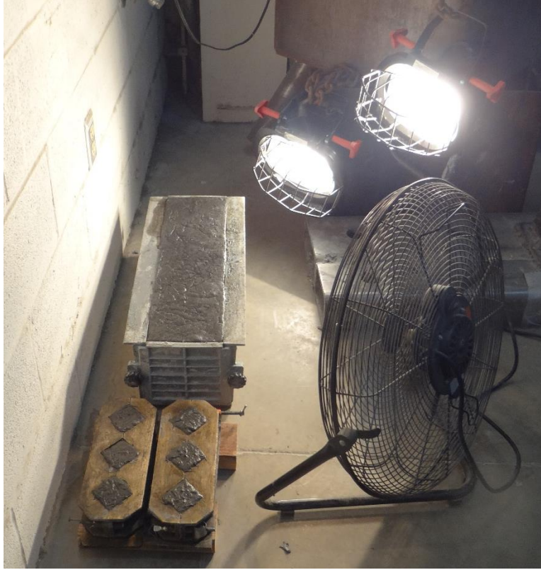
Figure 3.96 Specimens Subjected to Air and Heat (Simulation of external worst environment)
