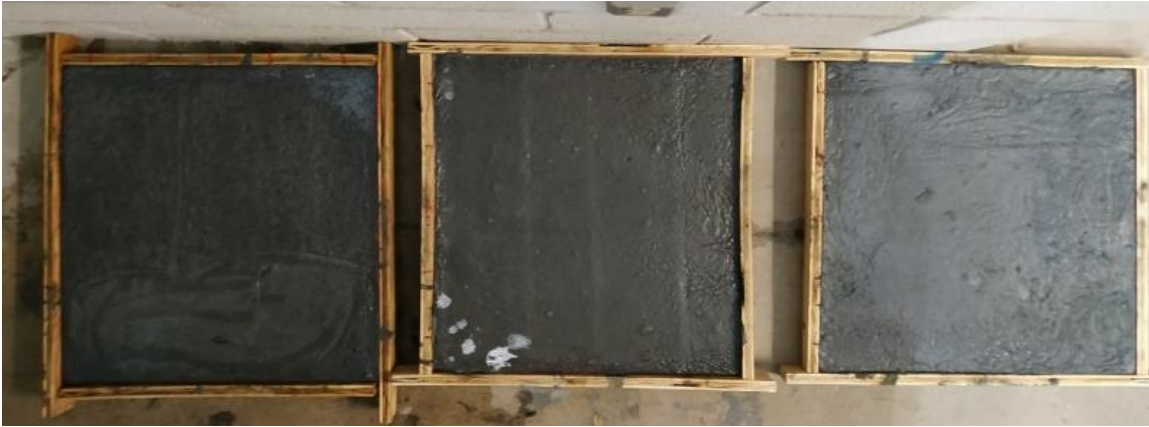
Figure 3.101 UHP-FRC Panels After 48 Hours: (a) No Curing, (b) Moisture Curing (c) Spraying with Concrete Curing Compound
