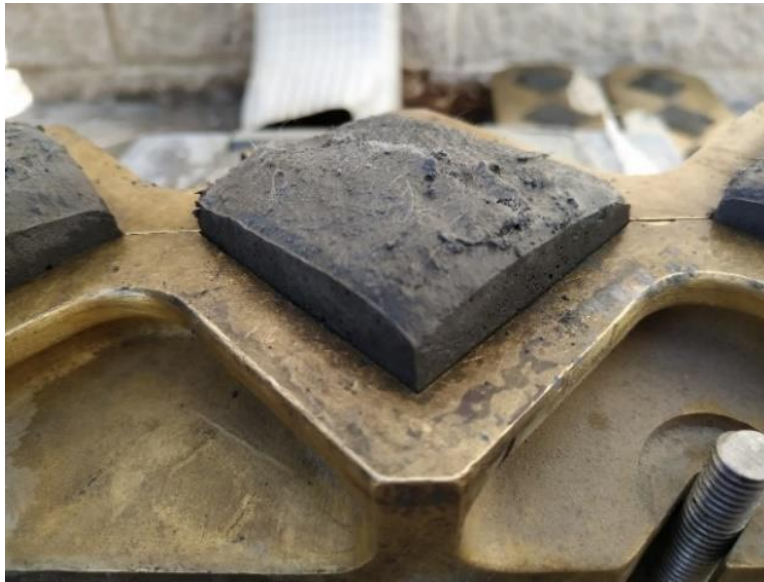
Figure 3.98 Swelling of UHP-FRC (a) UHP-FRC Cubes
