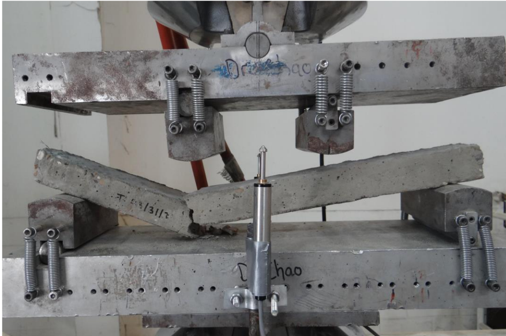
Figure 3.23 3 rd Point Bending Testing of Conventional Plain Concrete Beam
