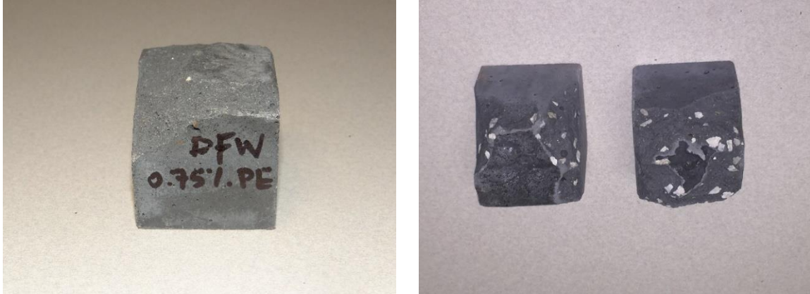
Figure 3.116 (a) Spalling of UHP-FRC Mix 6 (b) Spalling of UHP-FRC with Coarse Aggregates (mix 11)
