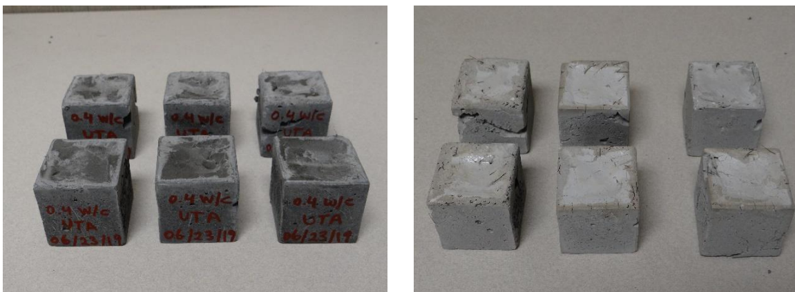
Figure 3.120 UHP-FRC with High w/cm Subjected Repetitive Temperature Change, w/cm 0.4, mix 15, before and after the Repeated Heating
