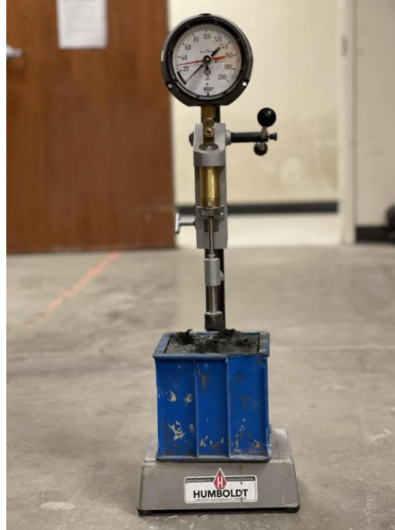
Figure 3.12 Proctometer to Determine the Yield Stress
