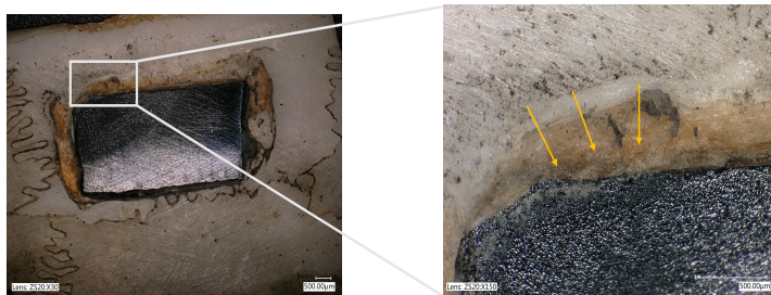
Figure 5.3. Reflective microscopic image of the implant-bone interface showing new bone growth (yellow arrows) on the SiONx coated implant.
