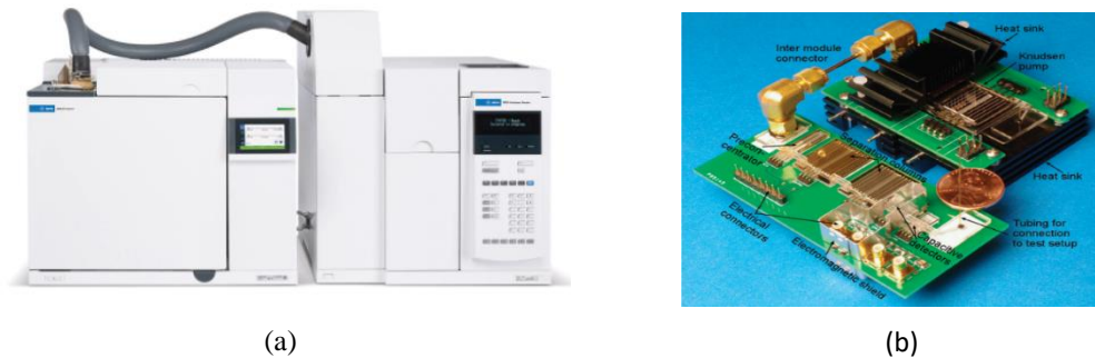
Figure 1-2 An example of (a) benchtop Commercial GC system (Agilent 8860) (b) \mu GC system [2]
