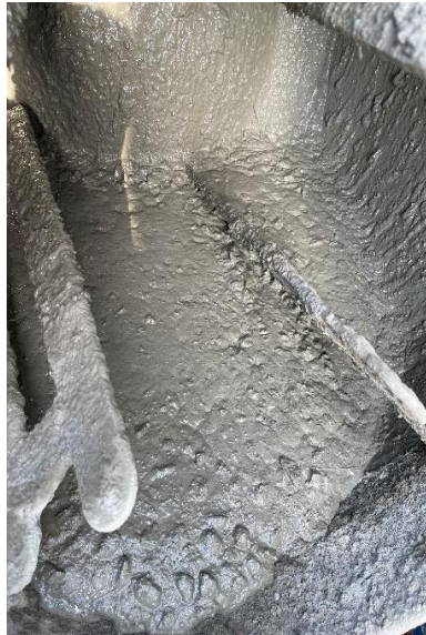
Figure 22: Images from casting day: a) Measured raw materials; b) Raw materials added to the drum mixer; c) Glass pozzolan added to the drum mixer; d) Mixing of concrete; e) Final concrete after mixing
