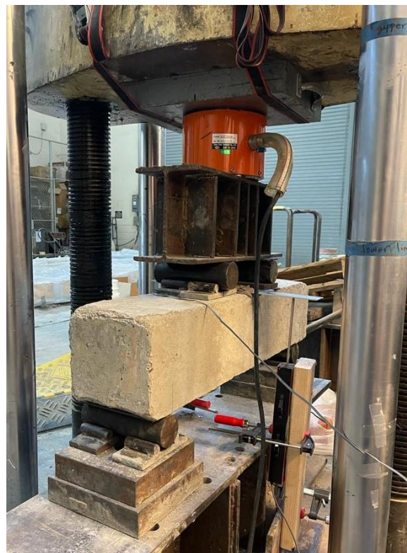
Figure 32: Flexural test setup with beam
