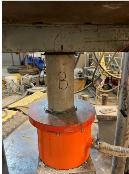
Figure 29: Compressive strength test setup
