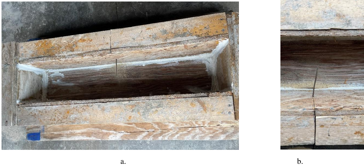
Figure 20: Set up of thermocouple in the formwork: a) Fixed thermocouple; b) Close shot
