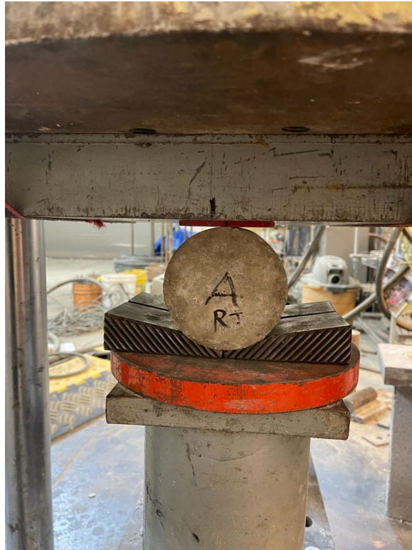
Figure 30: Split Tensile Strength test setup
