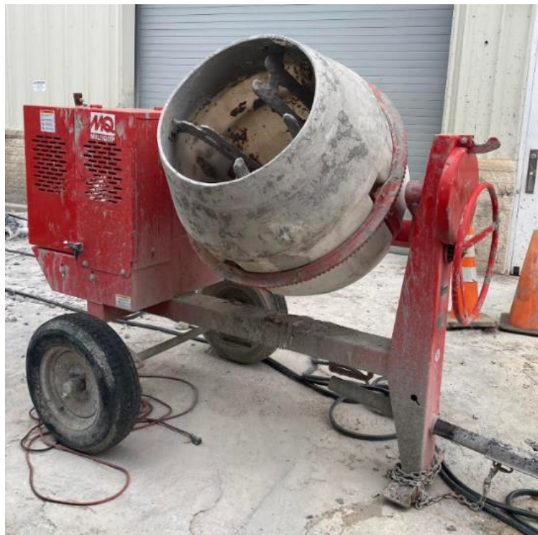
Figure 21: Drum mixer used for mixing concrete
