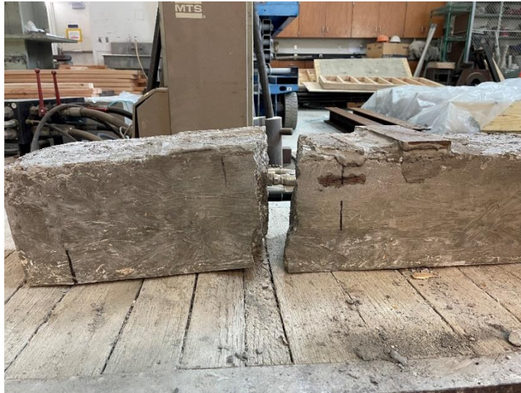
Figure 55: Beam failure pattern after flexure test
