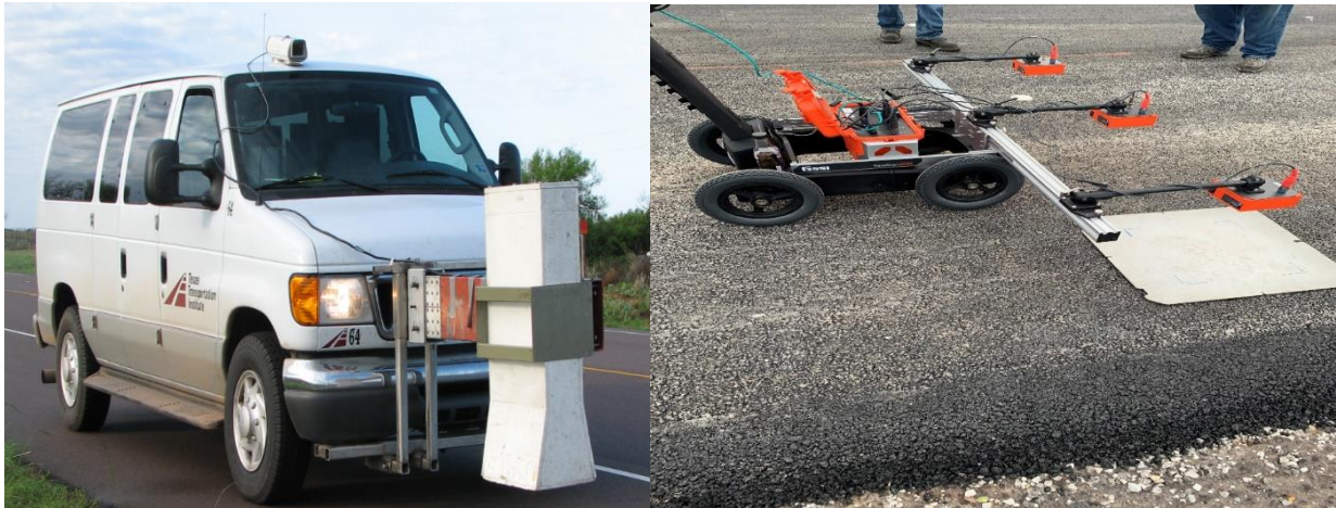
Figure 3.30 GPR with 1.0 GHz Horn Antenna and GPR with 3 Channel Rolling Density Meter
