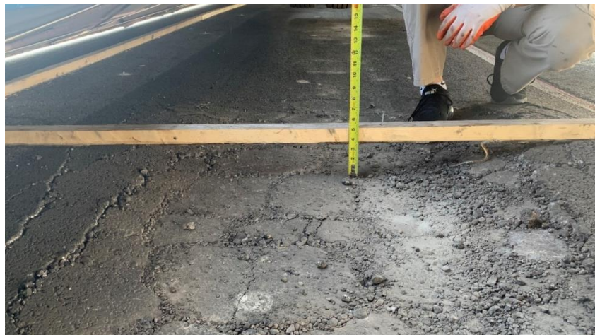
Figure 4.22 Rut depth measured on lane Q
