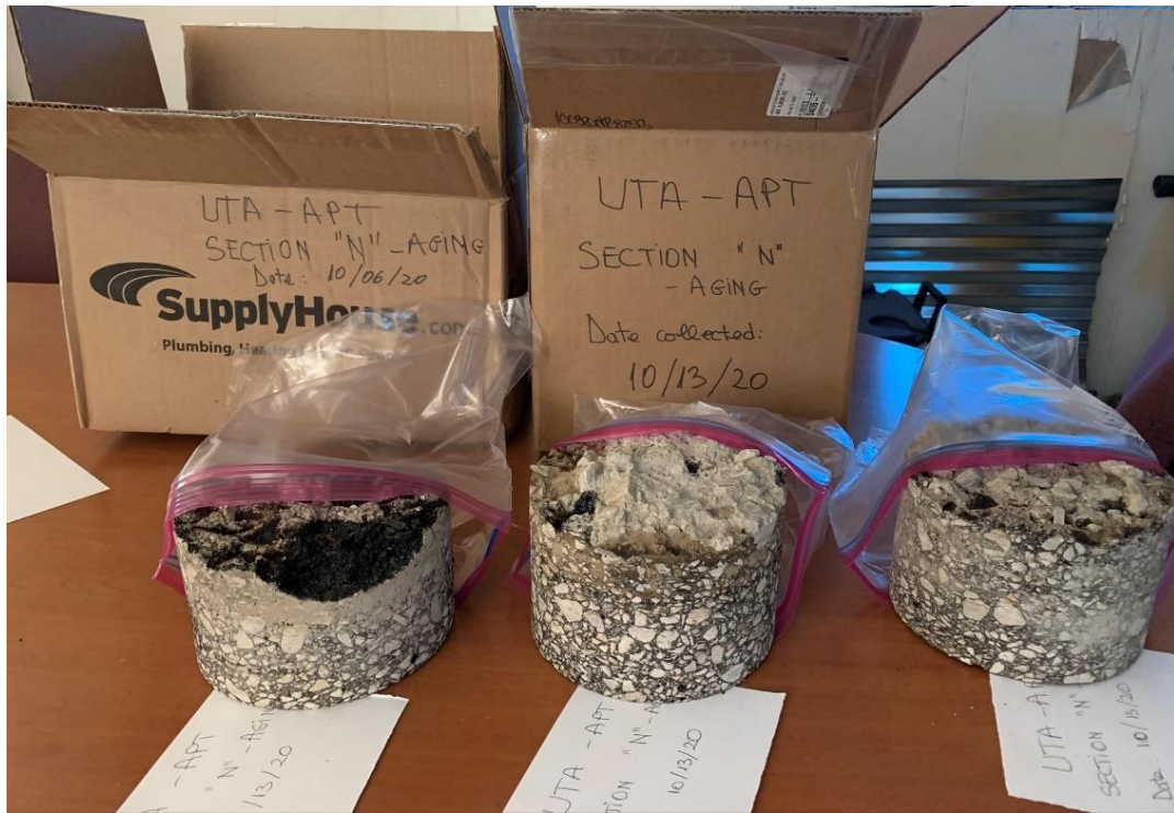
Figure 3.39 Extracted cores after 3 weeks of artificial aging
