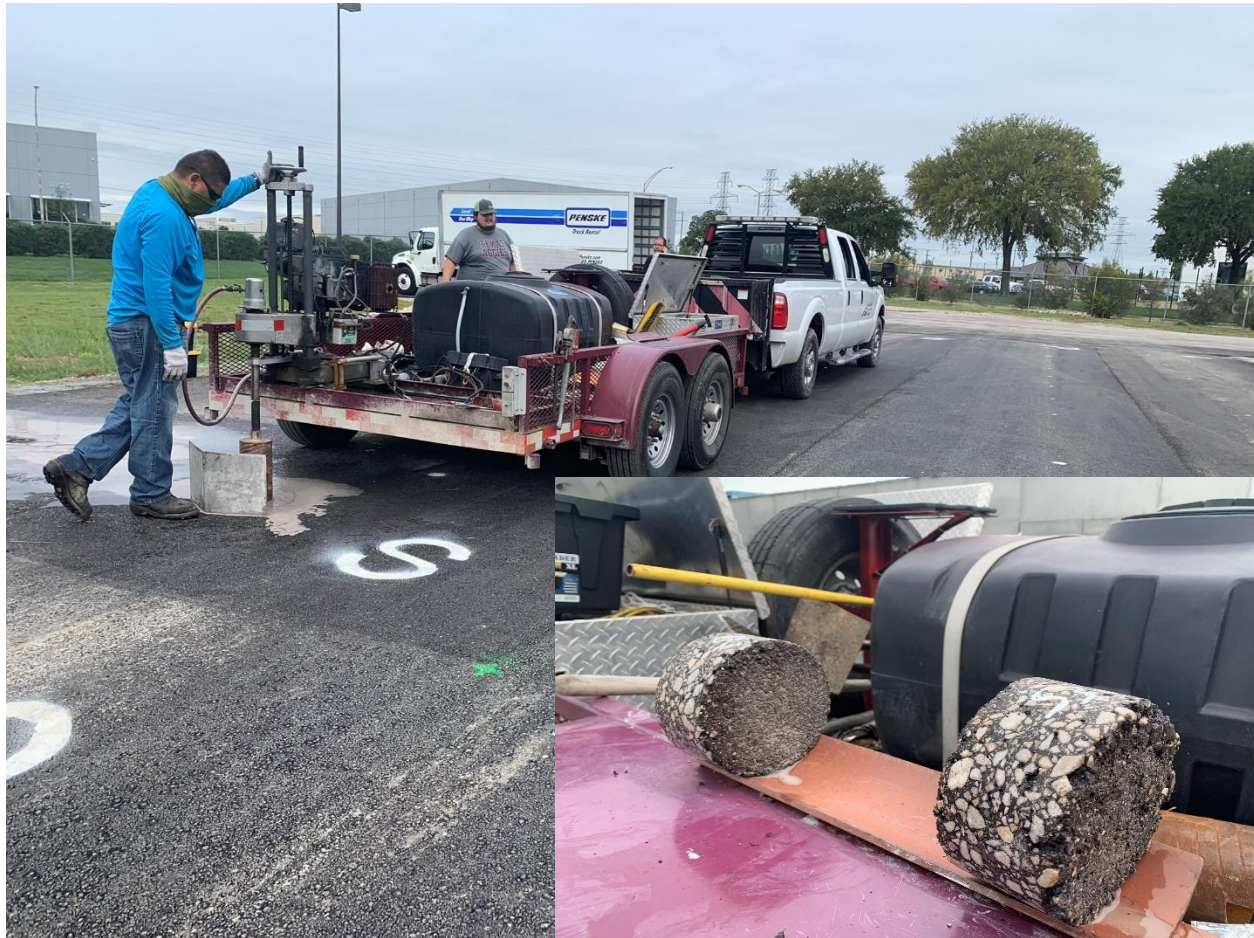
Figure 3.29 TTI extracting cores from Section S
