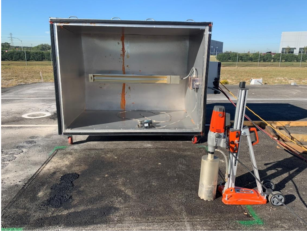
Figure 3.38 Coring after 4 weeks of artificial aging
