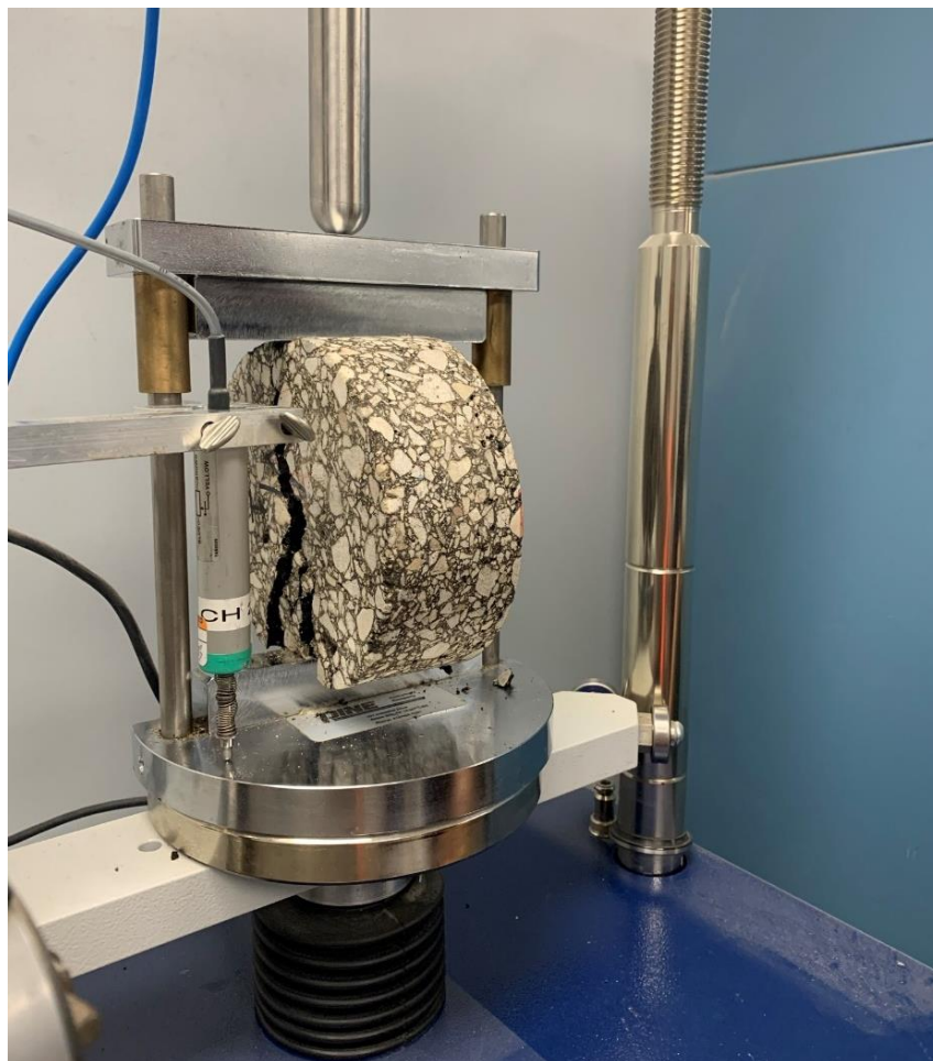
Figure 4.33 Testing setup for the IDEAL-CT Test
