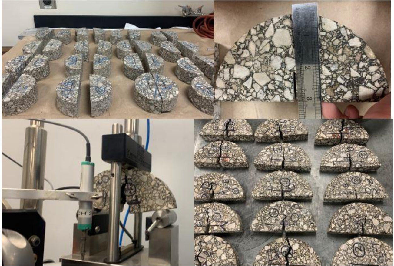
Figure 4.37 SCB Test setup and failed specimens
